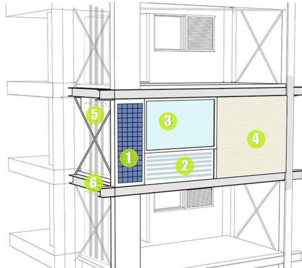
**Figure 3.** Exoskeleton (GET system) layout per housing unit during CDS: 1. Photovoltaic surface; 2. Opaque envelope; 3. Transparent envelope; 4. Flexible façade system; 5. Housing system installation; 6. Main supporting structure.
