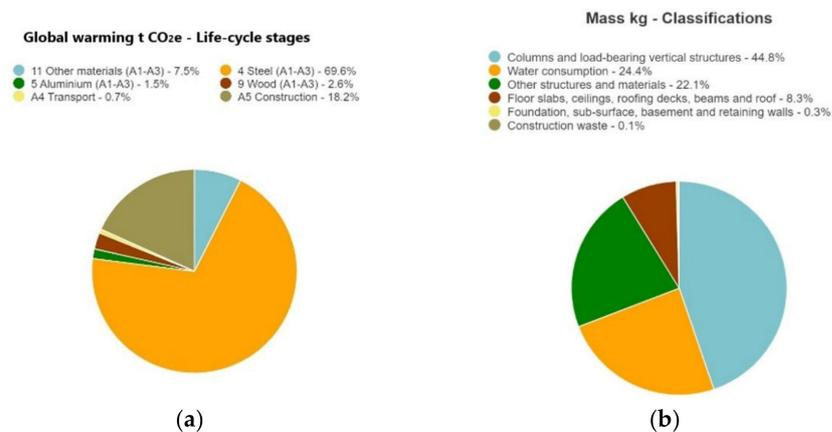
**Figure 13.** (a) Percentages of GWP (tCO<sub>2</sub>eq) emissions by life cycle stage; (b) Percentage of mass (kg) per construction component.
