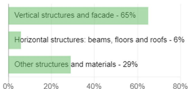
**Figure 9.** Percentage of embodied carbon stored in different parts of GET system.
