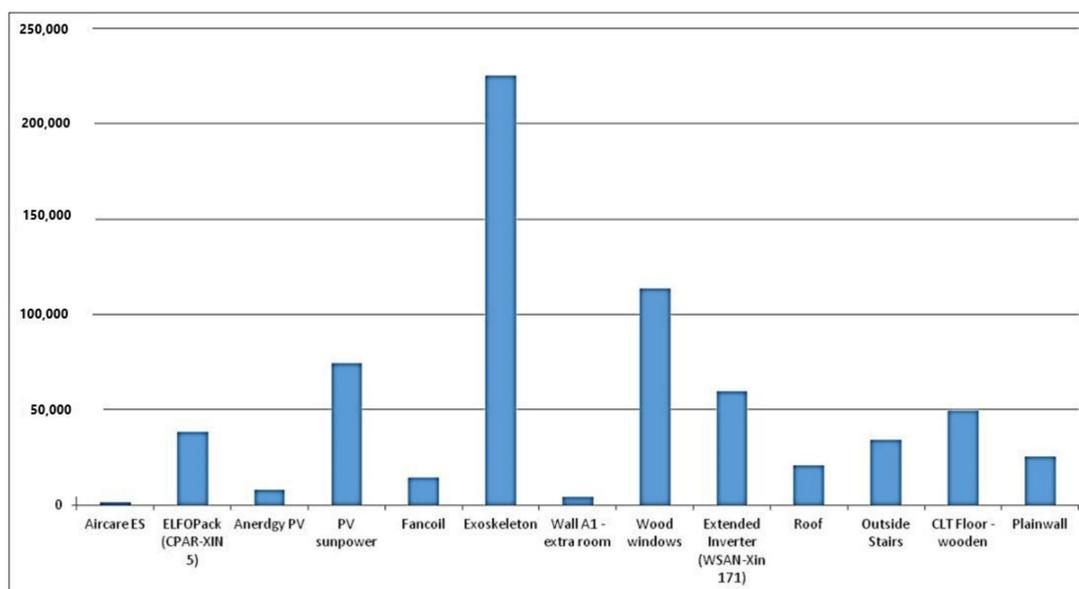
**Figure 8.** Impact of total components of the GET system [kgCO<sub>2</sub>eq] for a period of analysis of 50 years.
