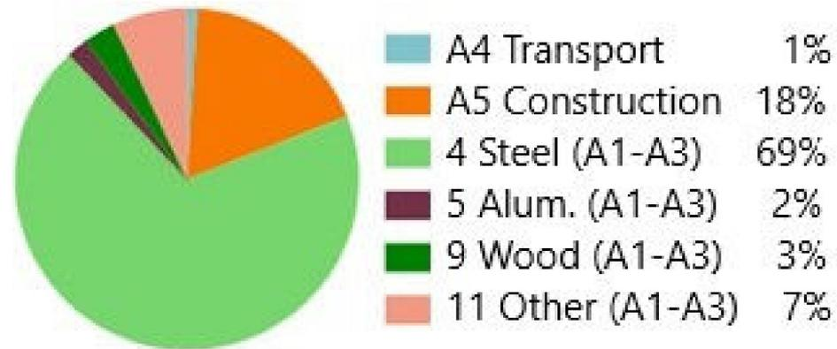
Figure 10. EC in life cycle phases A1–A5 (without foundations and demolition of balconies).
