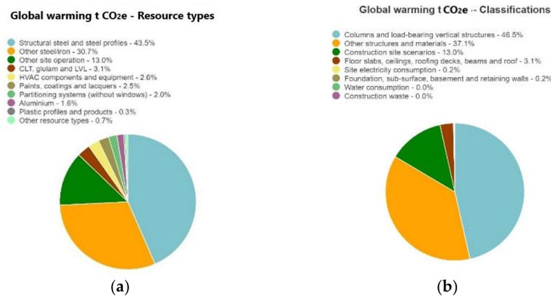
**Figure 12.** (a) tCO<sub>2</sub>eq emissions by resource type; (b) tCO<sub>2</sub>eq emissions per construction component.
