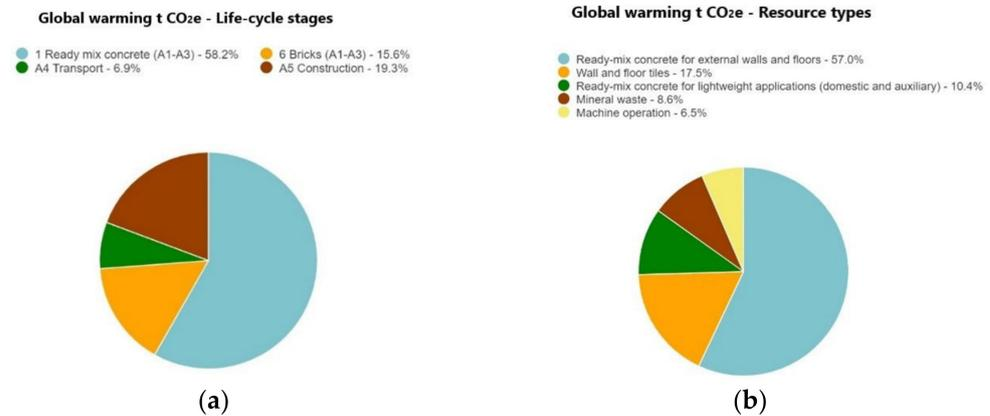
**Figure 14.** (a) Reinforced concrete: percentage of  $\text{kgCO}_2\text{eq}$  emissions by life cycle stage. (b) Reinforced concrete: percentage of  $\text{kgCO}_2\text{eq}$  emissions by resource type.
