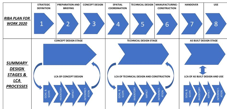
**Figure 4.** Sequence of design stages of the designing process from RIBA 2020 Plan of work [27] and comparison with summary design stages and LCA estimates.
