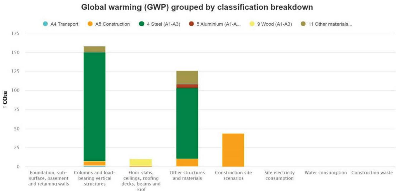
Figure 11. Global Warming GWP by classification breakdown in life stages A1–A5.
