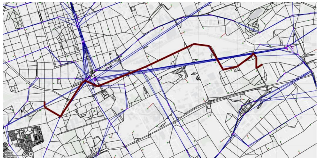
Figure 4. Directed graph with exemplary shortest path (dark-red edges) between two points. Black edges represent footways; blue edges represent rail and bus routes between purple-illustrated stations; green points represent the middle of traffic cells.
