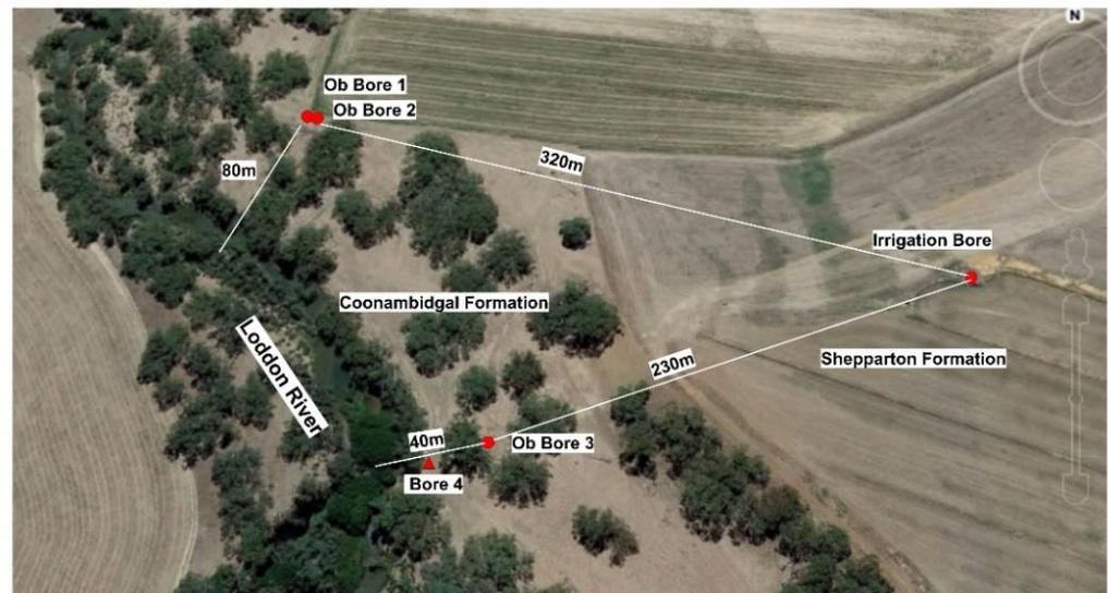
**Figure 25.** Location of observation bores (OB1–screen 13–9 m; OB2 and OB3–screens 5–6 m); stratigraphic bore (Bore 4); and extraction bore (screen 45–70 m). The strip eucalypt forest is a Terrestrial GDE tapping groundwater in the 9 m thick Coonambidgal Formation.
