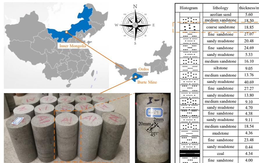
Figure 1. Project location map and prefabricated crack specimens.
