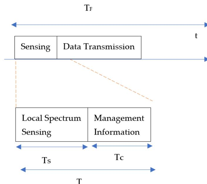
Figure 4. Spectrum sensing time representation.
