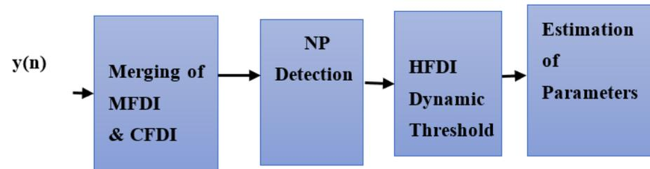
Figure 3. HFDI Spectrum Sensing Technique.
