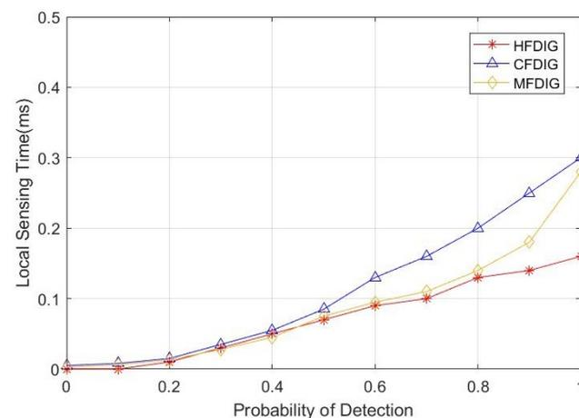
**Figure 12.** Local sensing time versus probability of detection at SNR =  $-10$  dB.
