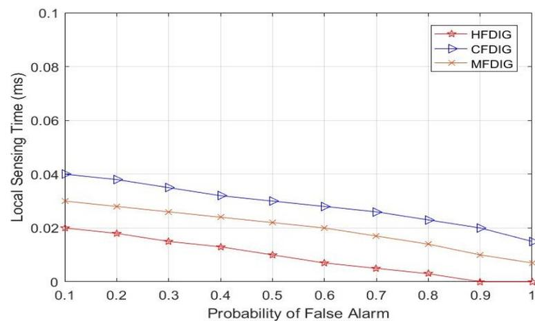
**Figure 11.** Local sensing time versus probability of false alarm at SNR=  $-10$  dB.
