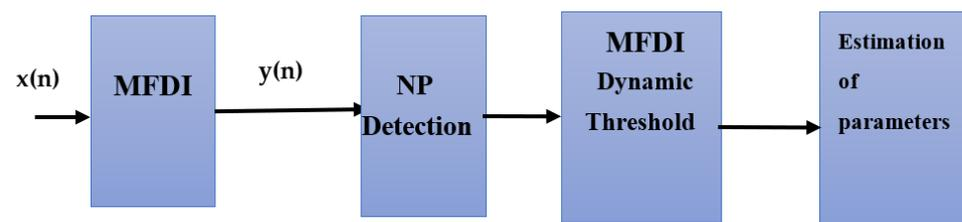
Figure 1. MFDI spectrum sensing technique.
