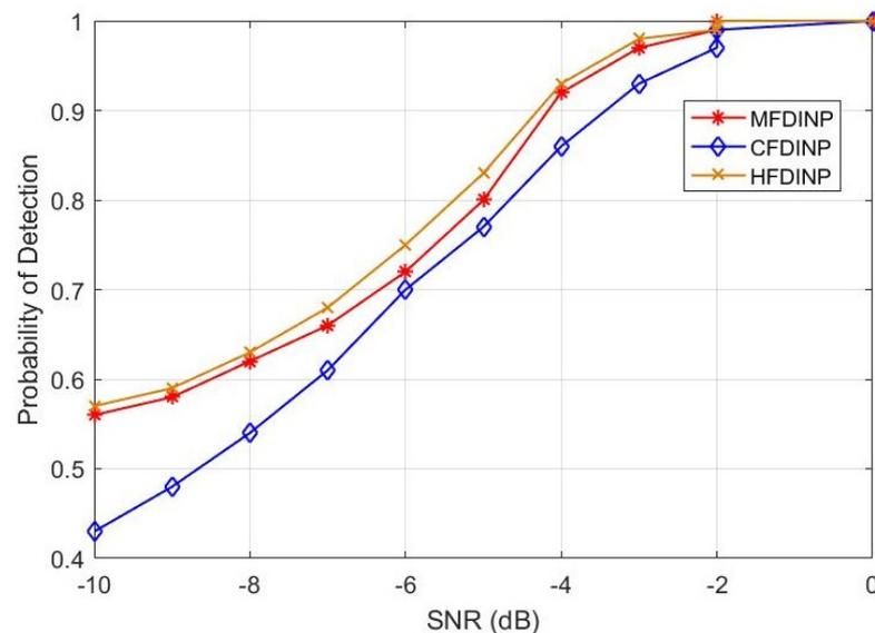
Figure 5. Comparison of  $P_D$  vs input SNR.
