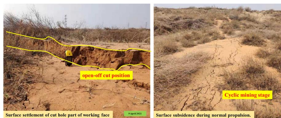
**Figure 10.** Comparison of surface subsidence between cut hole position and normal mining.
