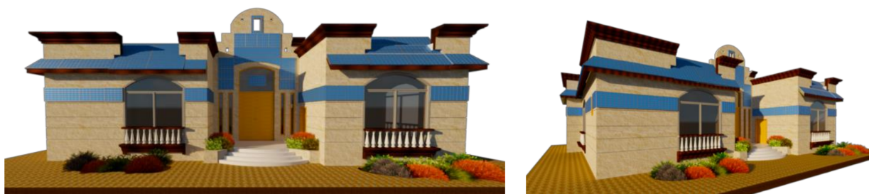
Figure 3. The 3D BIPV BIM model of the selected model house after integrating the solar panels.
