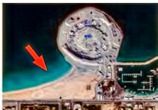
Figure 2. Interruption in natural sediment drift: the red arrow on the left indicates the increased sedimentation that might modify the natural shape of the shoreline (Source: Umm Suqeim 2 Harbor 25°09′08.01″ N and 55°11′50.46″ E) [47].
