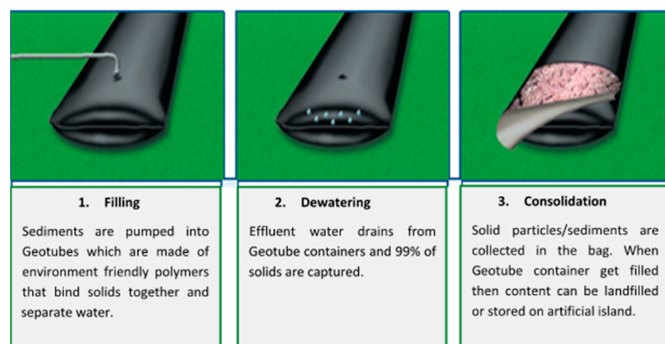
Figure 8. Mechanism of the geotube sediment filling, dewatering, and consolidation [73].
