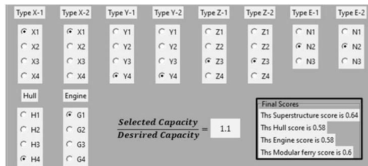
**Figure 10.** GUI for assembly of modular ferry. Vessel’s DPI is indicated on the right.
