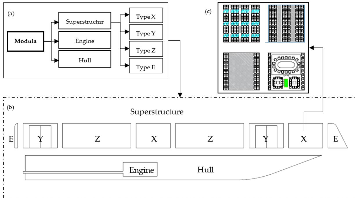
**Figure 8.** (a) Hierarchy of modular arrangement; (b) Representation of modular arrangement; and (c) An example of design alternatives for sub-module type Z of modular ferry.
