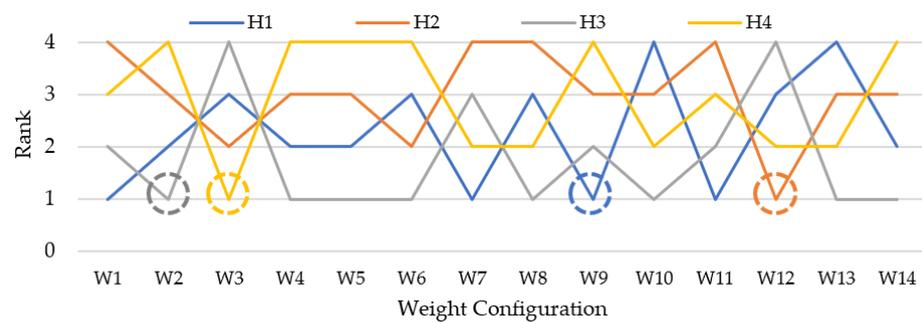
**Figure 11.** Sensitivity analysis shows the impact of different weight choices on the hull alternative's ranking. W1 refers to the choices made in Equation (18). W2 refers to the case where all sub-criteria have equal weights. In W3–W14, one sub-criterion is awarded a weight of 0.7, while others are equally distributed to 0.028. The order of assigning maximum weight is taken according to Table 2.
