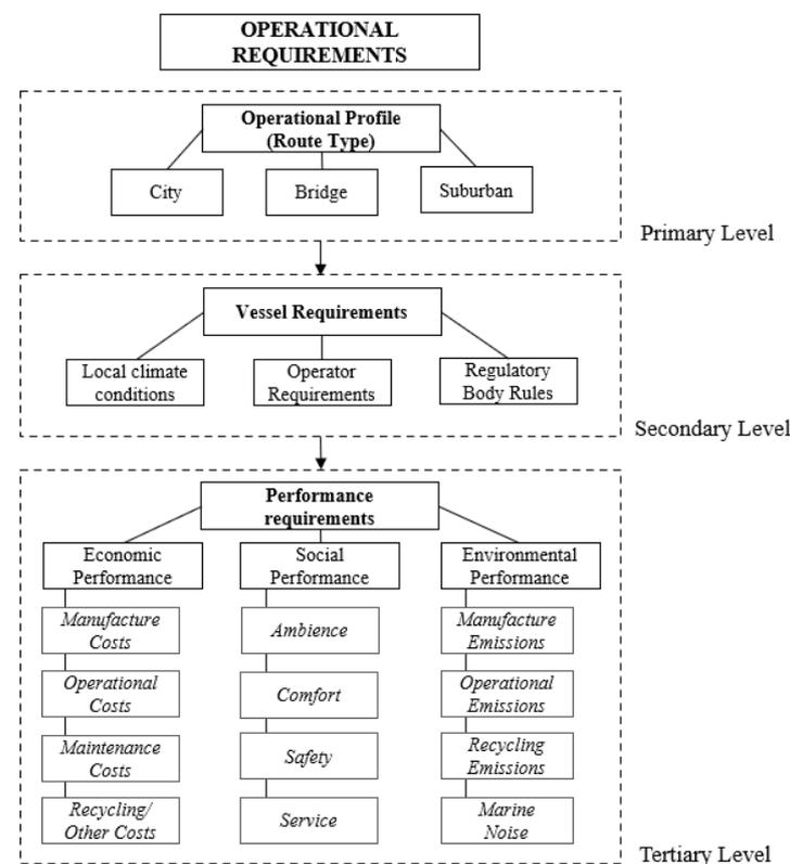
**Figure 1.** The operational requirements structure goes from broad to detailed design.
