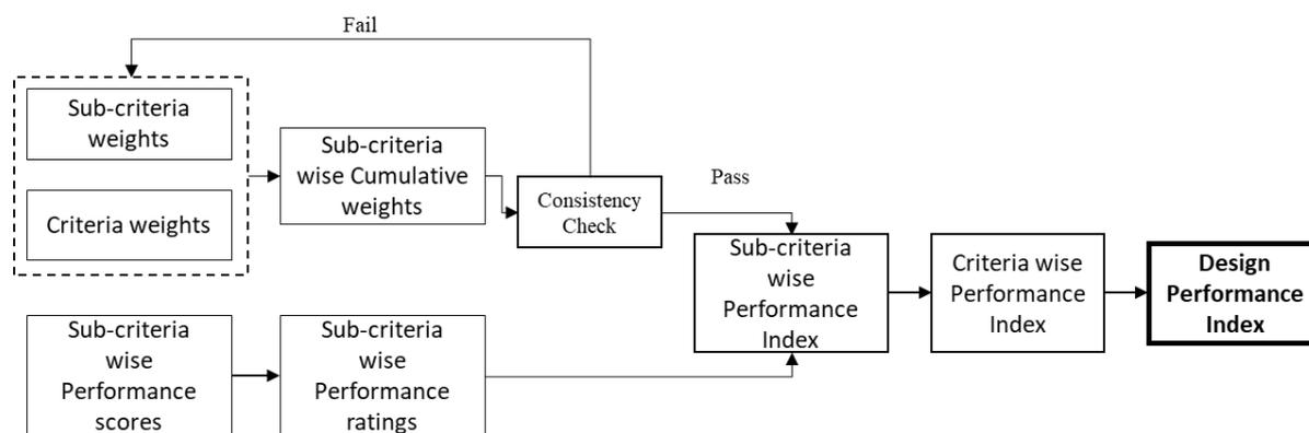
**Figure 2.** Methodology for evaluating the DPI of an alternative using AHP. Here, performance ratings represent normalized performance scores.
