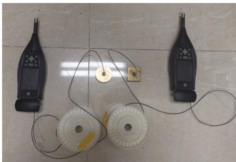
**Figure 1.** BK2270 two-channel noise and vibration analyzer (16.7–140 dB, 6.3–20,000 Hz).
