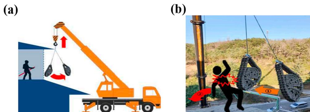
**Figure 6.** Hitting objects accident from mobile crane. (a) Schematic diagram of work at the time of the disaster and (b) schematic diagram of the situation at the time of the disaster.
