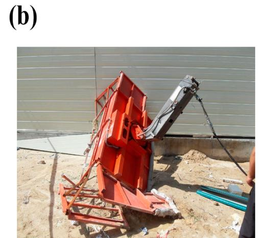
**Figure 4.** Falling accident from mobile crane. (a) Accident workplace and (b) falling due to breakout of the boarding equipment.
