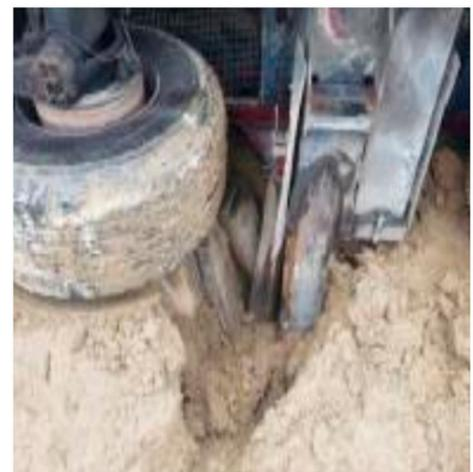
**Figure 5.** Overturning accident from mobile crane. (a) Mobile crane overturning accident and (b) outriggers more than 2 m into the ground.
