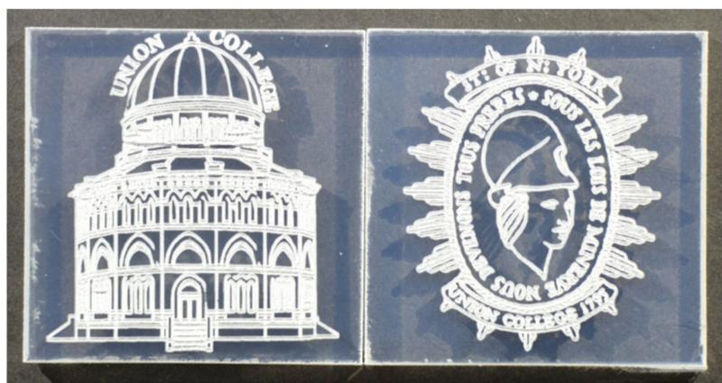
**Figure 11.** Photographs of  $5 \times 5 \times 0.5$  cm laser-cut and etched silica aerogel monoliths. These aerogel samples were photographed on top of black flocked paper.
