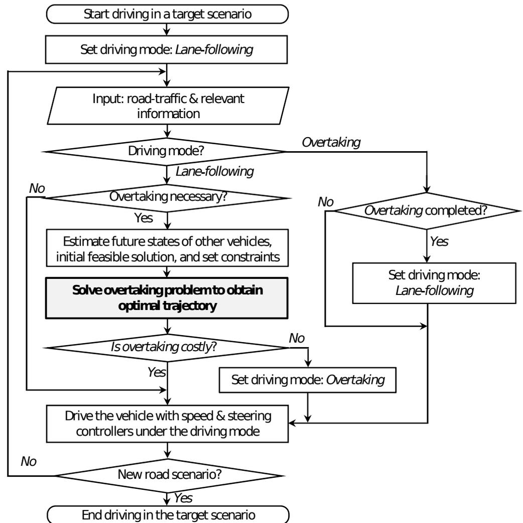
**Figure 3.** Flow chart of the proposed optimal trajectory generation scheme for autonomous overtaking in the driving framework.
