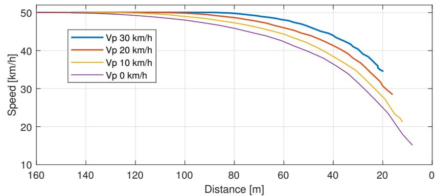
**Figure 6.** The speed of the host vehicle when approaching a slow preceding vehicle before attempting for lane change or overtake.
