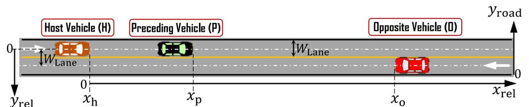
**Figure 2.** An overtaking problem of a host vehicle (H) with its original preceding vehicle (P) and an oncoming vehicle in the opposite lane (opposite vehicle). With the host vehicle's position  $x_h$  as the origin, the positive lateral axis  $y_{rel}$  is given according to the direction of the overtaking lane.
