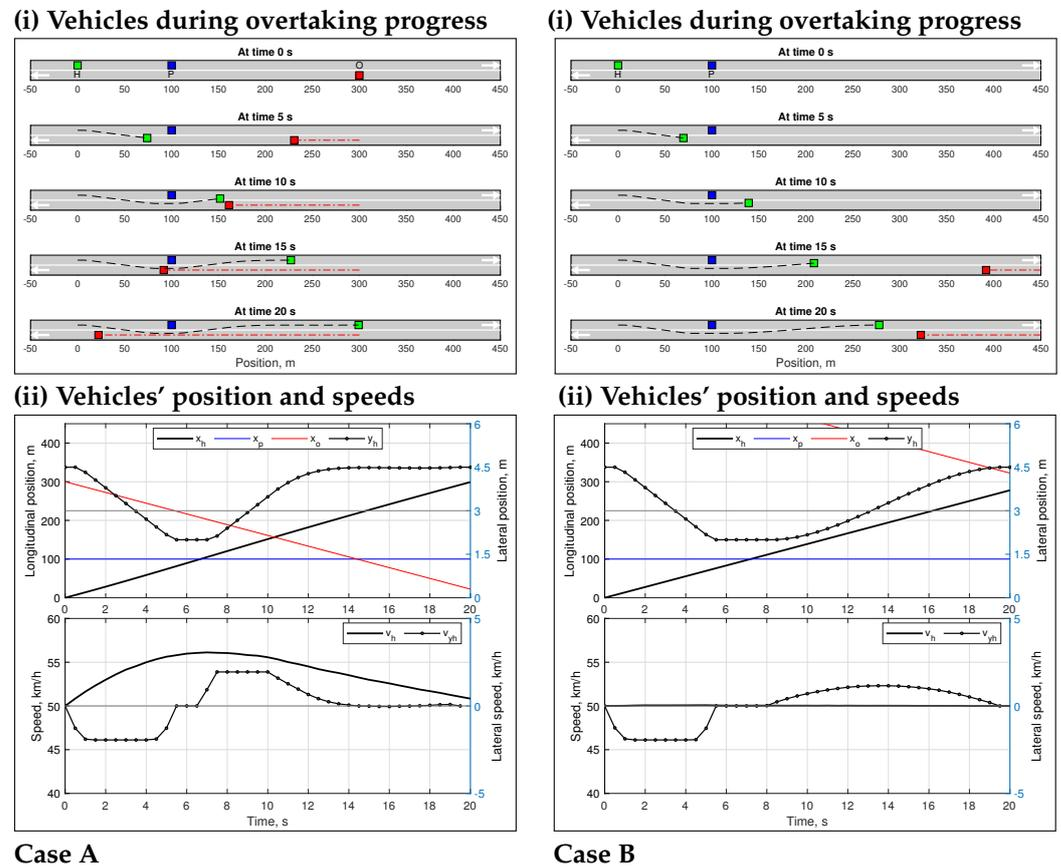
**Figure 4.** Two overtaking cases with preceding (P) vehicle with zero speed: (**Case A**) encountering an opposite vehicle (O) and (**Case B**) with a far opposite vehicle. In each case, (i) the vehicles' positions are shown at each 5 s during the overtaking course, and (ii) both longitudinal and lateral positions and speeds of the vehicles are illustrated using trajectories.
