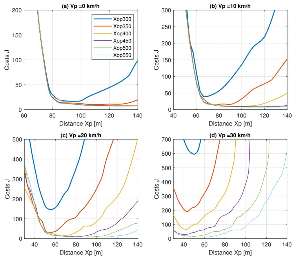
**Figure 7.** The overtaking costs with respect to the initial distance  $X_p$  to the slow preceding vehicle for various longitudinal gaps  $X_{op}$  between the preceding and opposite vehicles and speed of the preceding vehicle  $V_p$ . Legend is only shown in (a), for simplicity.
