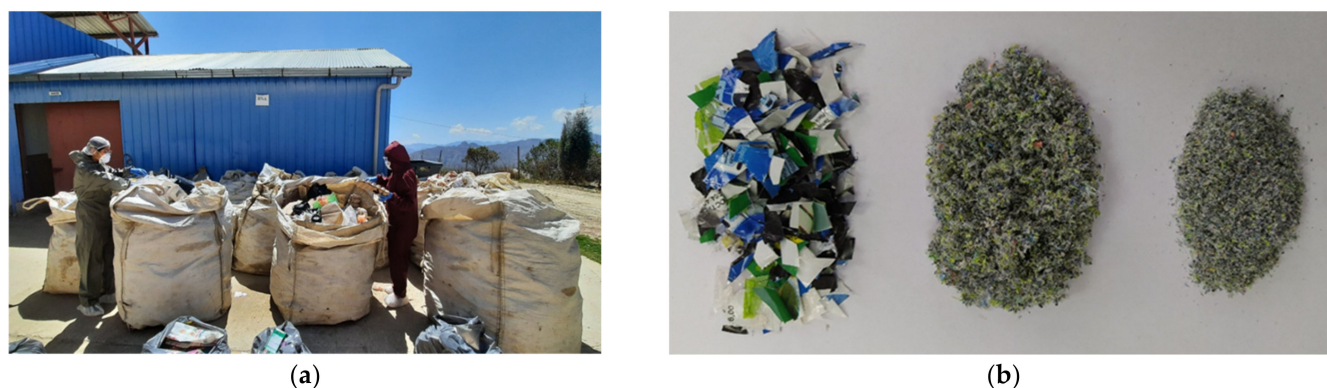
Figure 5. Sampling procedure of the rejected materials: (a) rejects collection from the MRF of La Paz; (b) shredded non-recyclable plastics for laboratory testing.
