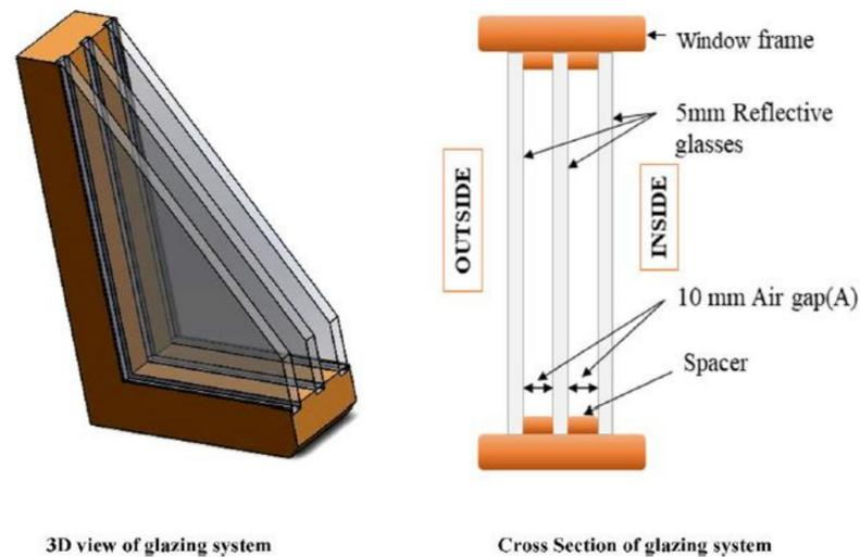
**Figure 8.** A triple-glazed window unit with reflective glasses. Adapted with permission from Ref. [48]. 2021 Gorantla et al.
