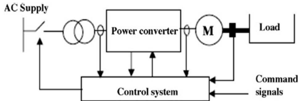
**Figure 13.** Basic components of a variable speed drive (VSD). Adapted with permission from Ref. [60]. 2012 Saidur et al.
