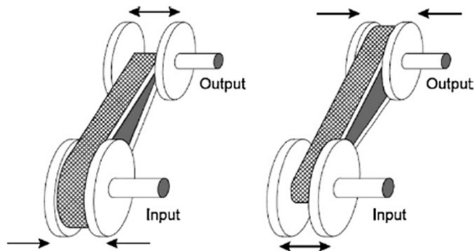
**Figure 12.** Adjustable sheave belt-type mechanism used in VSD. Adapted with permission from Ref. [60]. 2012 Saidur et al.
