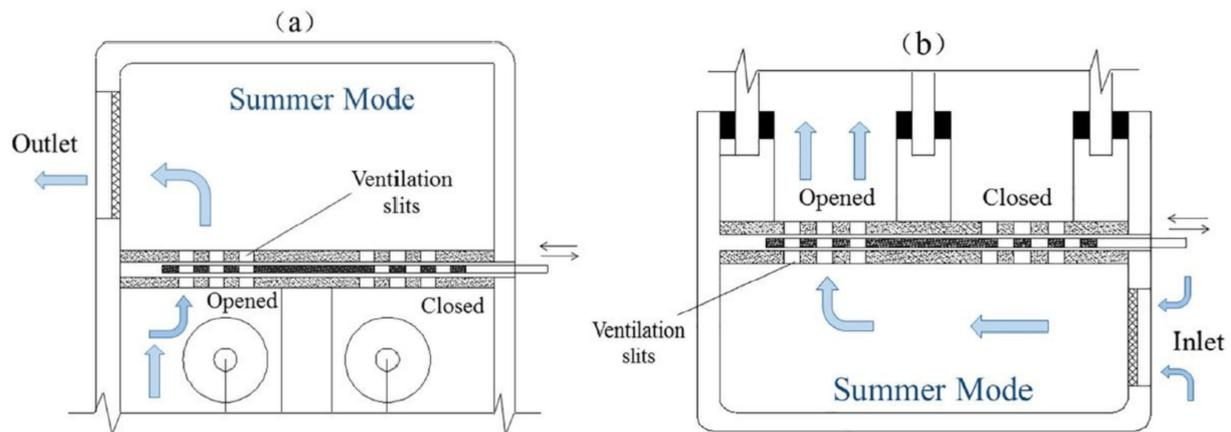
**Figure 10.** Switchable components of SEA window: (a) upper part, (b) lower part. Adapted with permission from Ref. [49]. 2016 Zhang et al.
