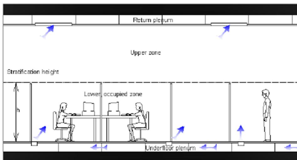
**Figure 6.** A schematic diagram of an underfloor air distribution system. Adapted with permission from Ref. [26]. 2013 Kim et al.
