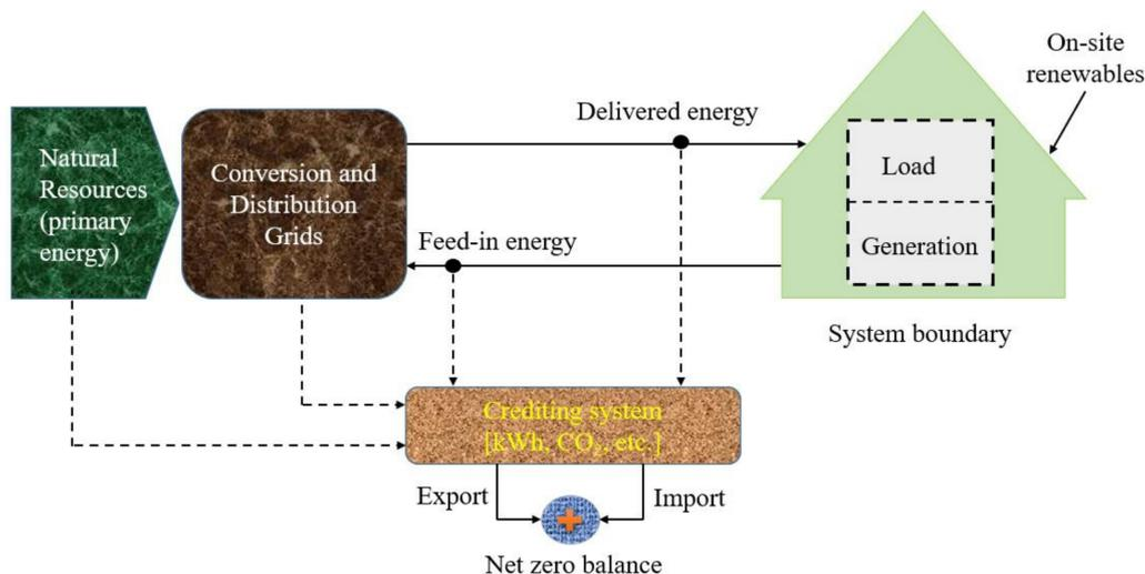
Figure 5. Schematic diagram of a typical net-zero energy building [17].
