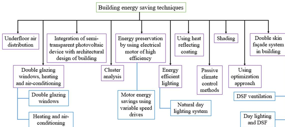
Figure 4. Building energy-saving techniques at a glance [14–16].
