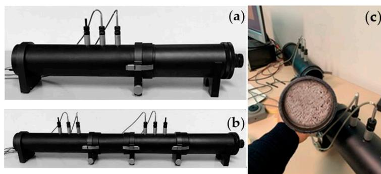
**Figure 3.** Impedance tube: (a) absorption and (b) TL measurements configurations; (c) Khorasan wheat chaff sample in the tube.
