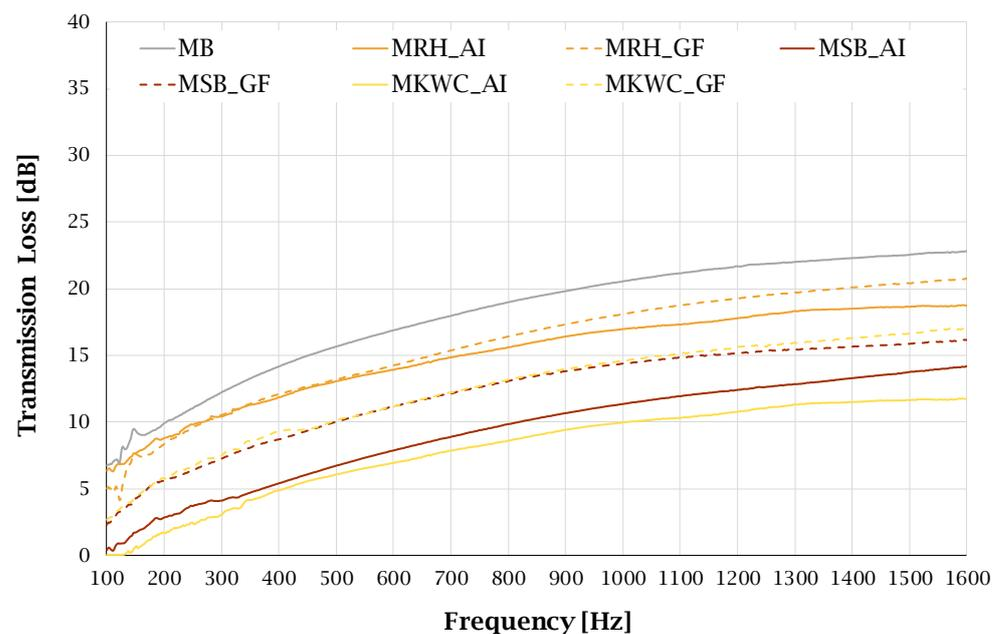
Figure 6. Normal incidence TL of the samples.
