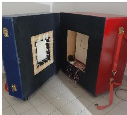
**Figure 2.** Small Hot Box apparatus.
