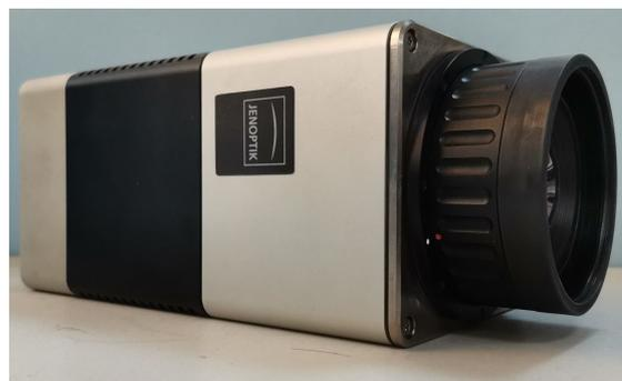
**Figure 4.** Infrared thermal imager.
