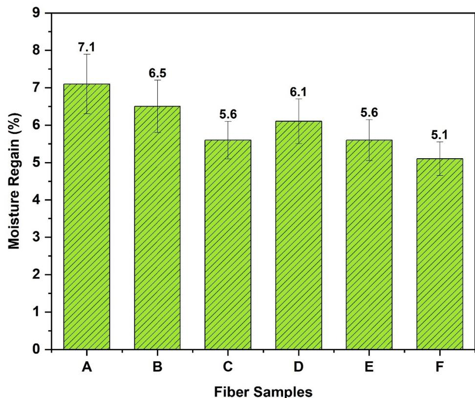
Figure 2. Comparison of moisture regain of developed fiber samples.
