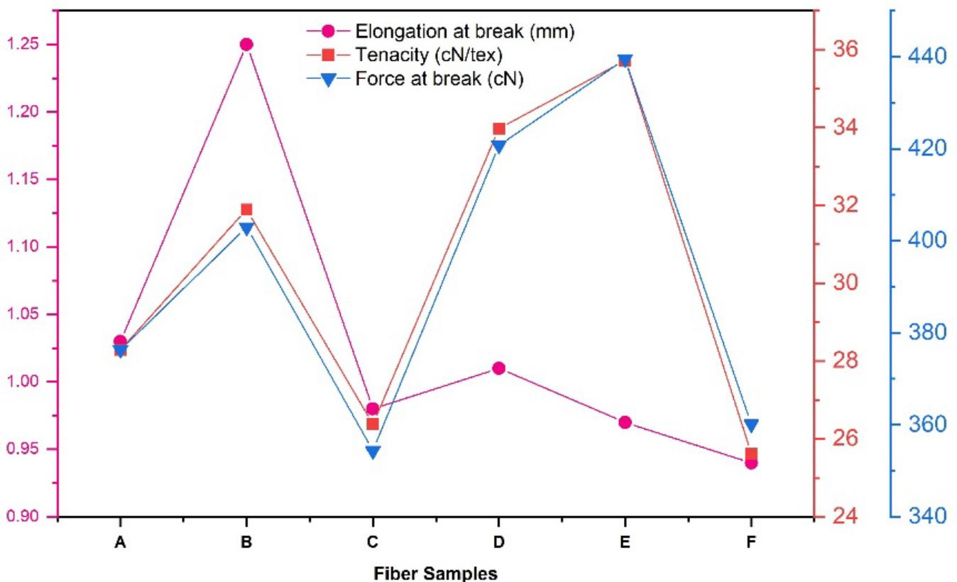
**Figure 3.** The variation of elongation at break, tenacity, and force at break of various fiber samples.
