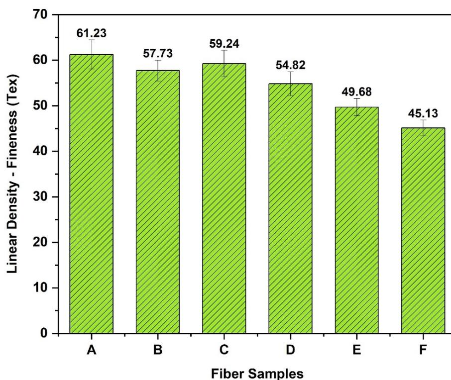
Figure 1. Comparison of fiber linear density of developed samples.
