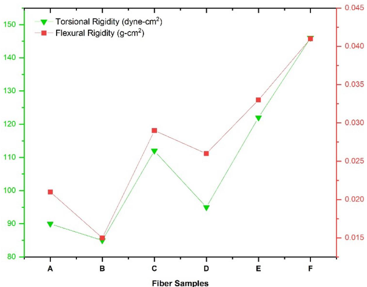
**Figure 4.** The variation of torsional and flexural rigidity of various fiber samples.
