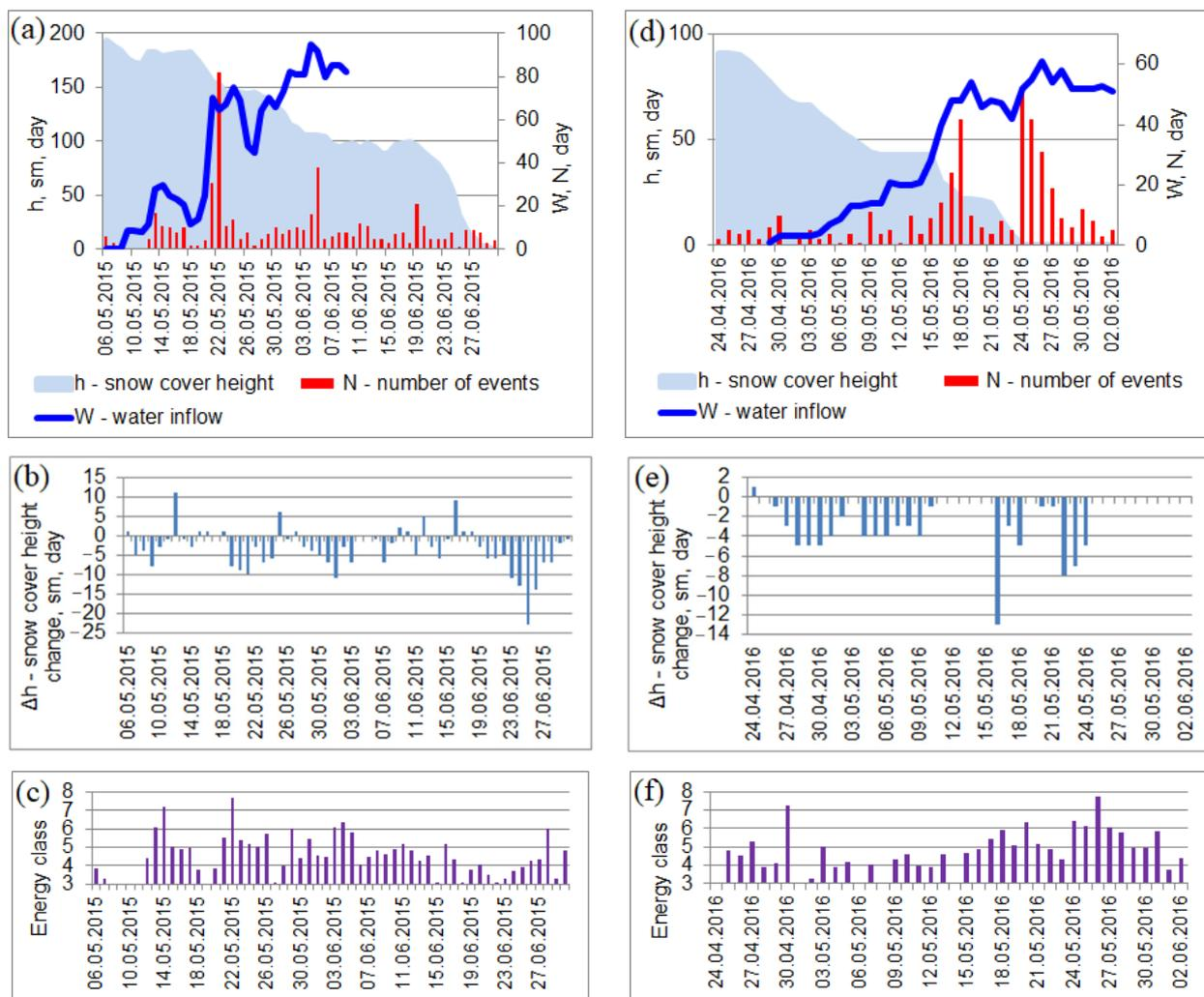
**Figure 7.** Influence of snow cover height and water inflow on seismicity changes. (a,d) the relationship of seismicity, water inflow, snow cover height; (b,e) snow cover height change; (c,f) energy class of seismic events change; (a–c) 2015 year; (d–f) 2016 year accordingly.
