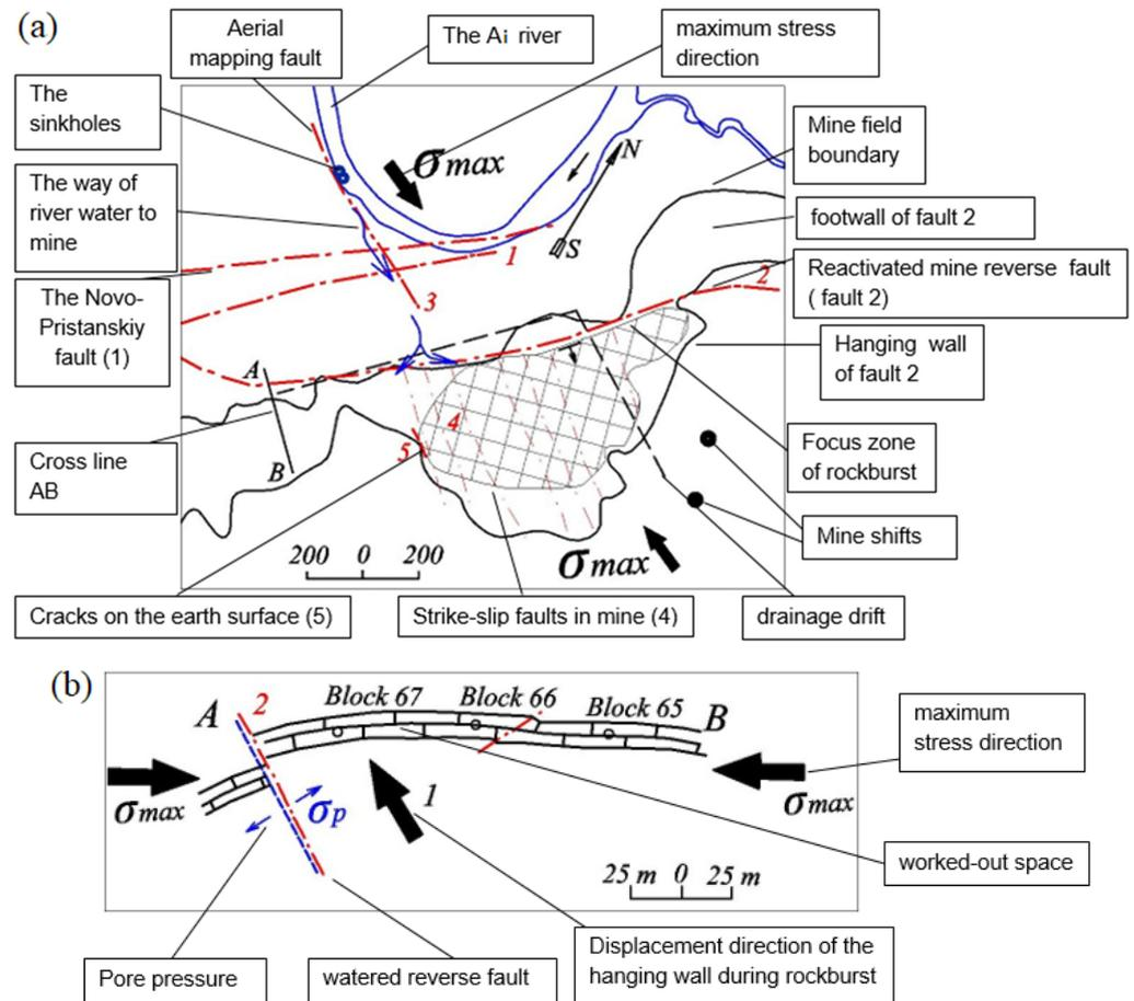
**Figure 9.** Tectonophysical diagram of the 28 May 1990, rockburst: Factual scheme of the bauxite deposit region (a); cross section along AB line (b) (according to (a)).
