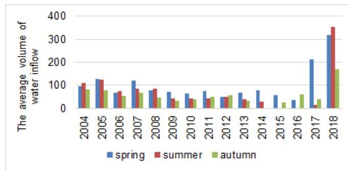
**Figure 3.** Average daily water inflow ( $\text{m}^3/\text{day}$ ). The measurements were performed in the junction area of the Rasvumchorr underground mine and the Tsentralny open pit. There are no data on water inflow measurements during the summer period of 2015–2016.
