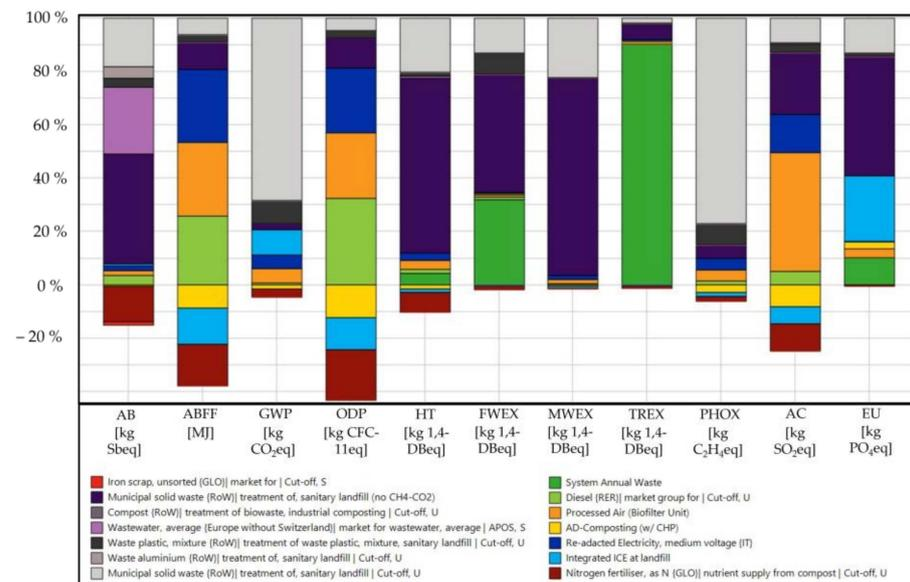
**Figure 4.** Results of the LCA for the facility under investigation (colours represent the different subprocesses).
