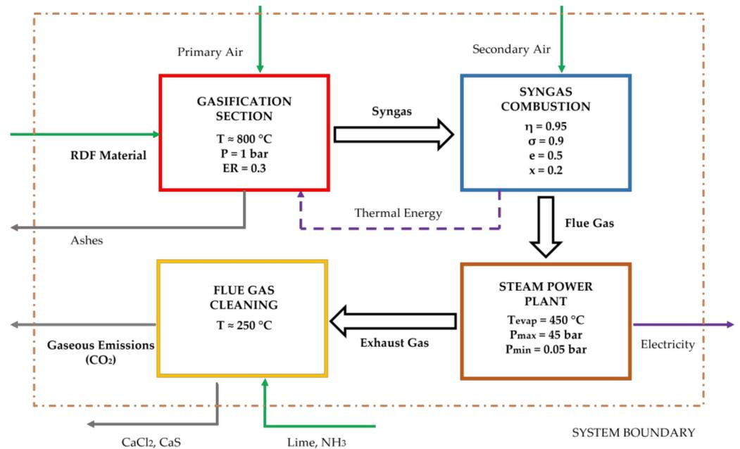
Figure 15. Process diagram of the gasifier combined with the steam power plant unit.
