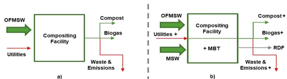
**Figure 2.** Material and energy flows in a standard composting facility, (a); Material and energy flows in a composting facility implementing MBT, (b).
