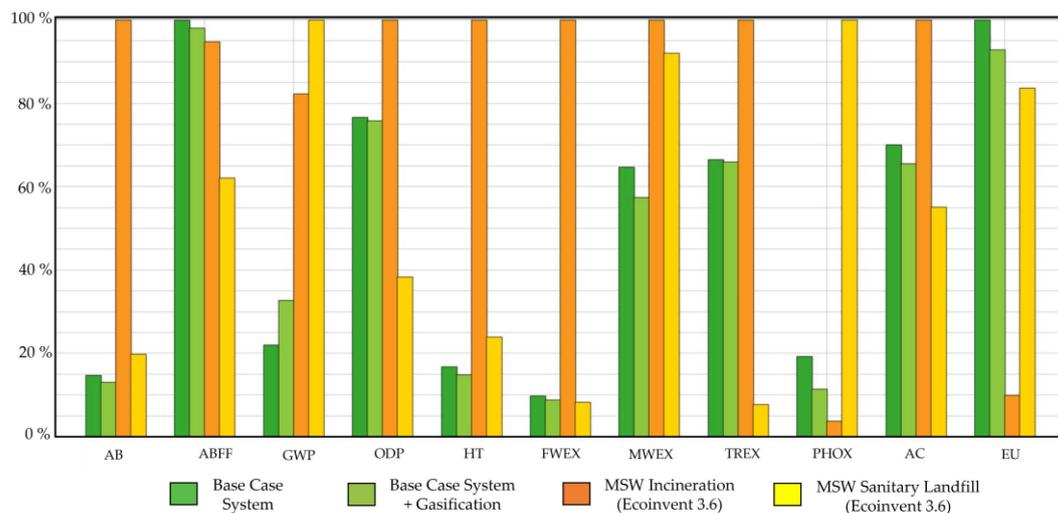
Figure 16. LCIA of the facility integrated with the gasifier compared to incineration (orange) and landfilling (yellow).
