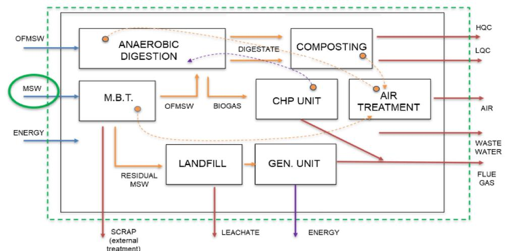
**Figure 3.** Detailed diagram of the material and energy flows in the analyzed domain (blue lines for energy and waste inputs, red for material outputs, violet for energy output and orange for internal flows).
