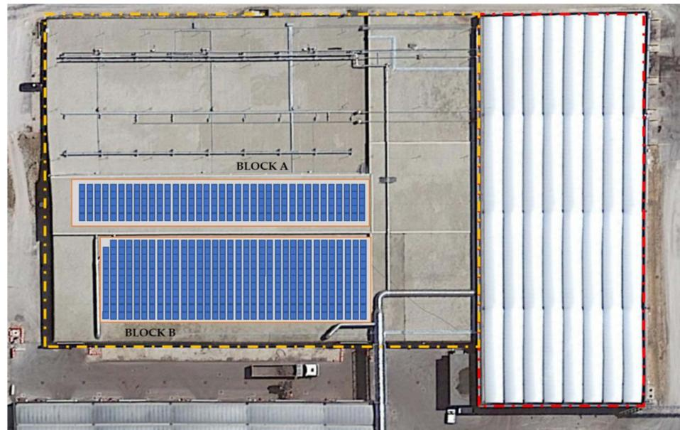
**Figure 12.** Top view of the proposed PV plant (dashed red lines represent the building area where the MBT is located, and yellow ones denote the perimeter of the digester section).
