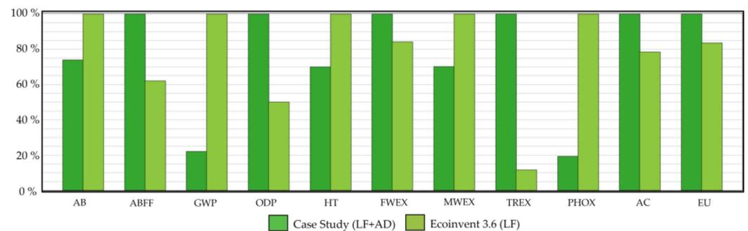
**Figure 8.** Comparison of the impact categories in the facility under investigation with those of a standard sanitary landfilling treatment process.
