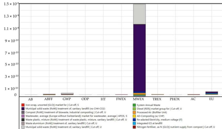
**Figure 5.** Normalization of the impact factors according to CML baseline method.
