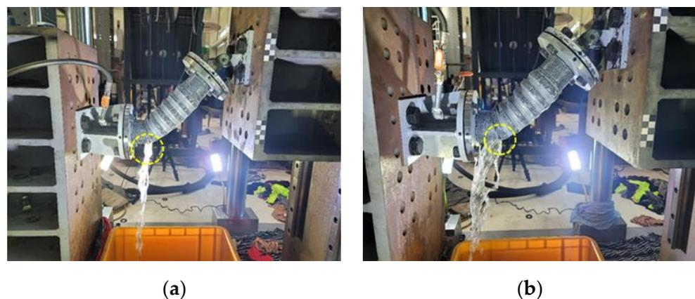
**Figure 7.** Leakage of monotonic bending tests: (a) 2-ply bellows, (b) 3-ply bellows.
