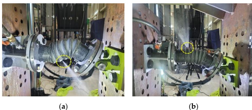
**Figure 9.** Leakage of constant amplitude cyclic bending tests: (a) 2-ply bellows specimen, (b) 3-ply bellows specimen.
