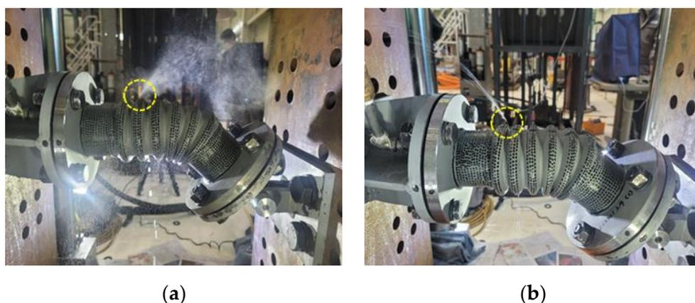
**Figure 8.** Leakage of multi-step increasing amplitude cyclic loading tests: (a) 2-ply bellows, (b) 3-ply bellows.
