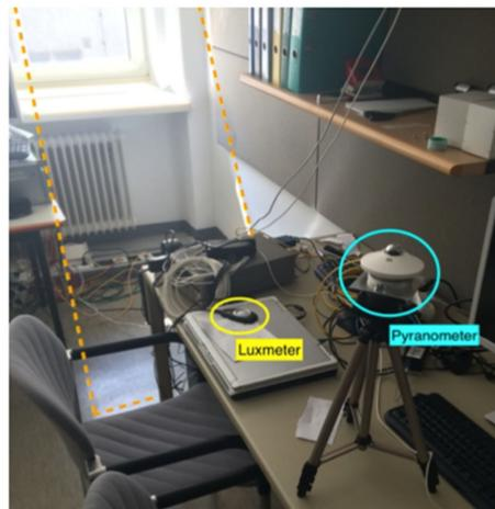
**Figure 18.** Measuring setup for lux meter and pyranometer and representation of the incidence of radiation in room B Z.12.
