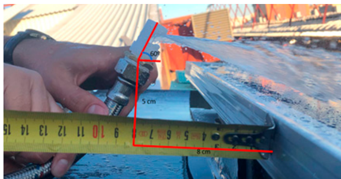
Figure 20. Optimal configuration of the nozzle.
