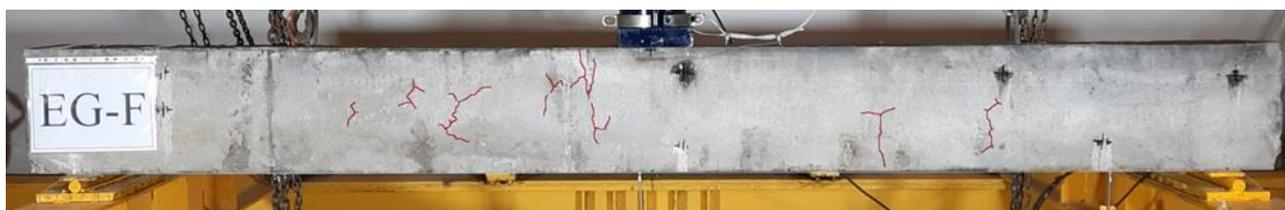
Figure 7. Thermal cracks during the fire loading.
