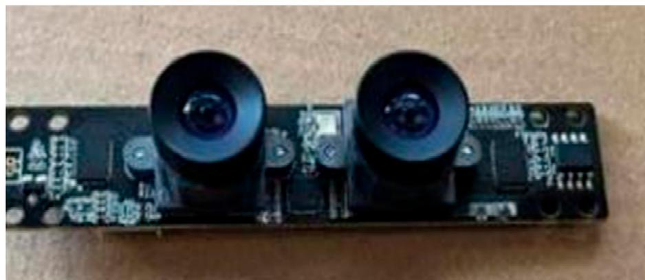
**Figure 12.** The binocular camera used in this experiment.
