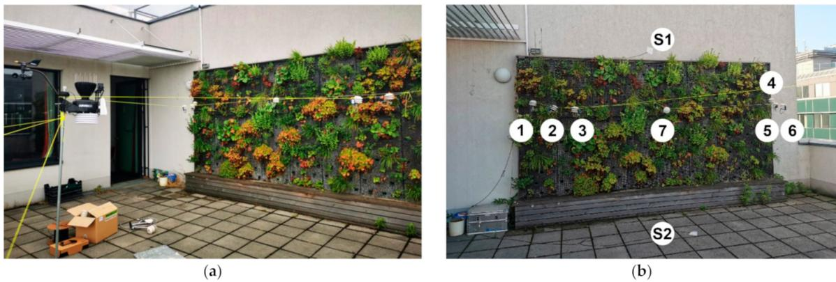
**Figure 3.** Images of the installation of the sensors at Diefenbachgasse School: (a) position of the weather station; (b) position of the temperature and humidity as well as surface temperature sensors.
