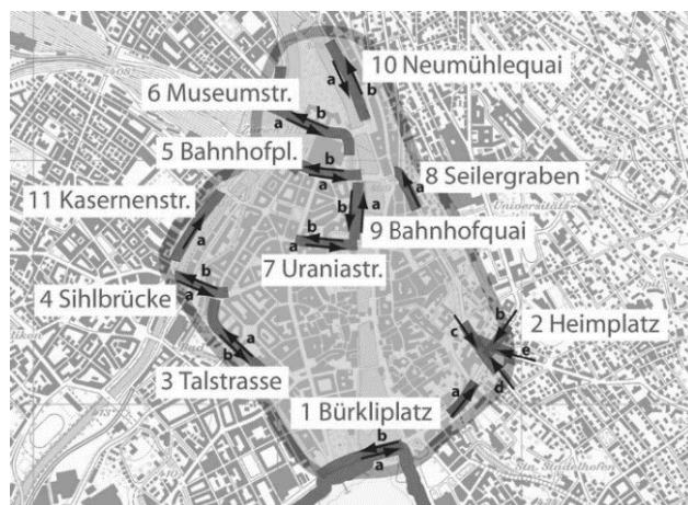
Figure 7. Map of the inner city of Zurich and the streets monitored by the Zurich model. Once a level of service reduction is detected, traffic lights on the city access roads generating the traffic for those inner streets are adjusted automatically Source: [62].
