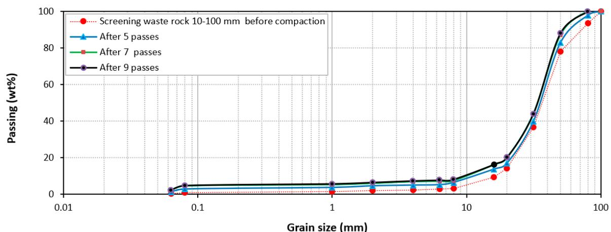
**Figure 7.** Evolution of grading curves of SWR (10–100 mm) according to the number of compactor passes.
