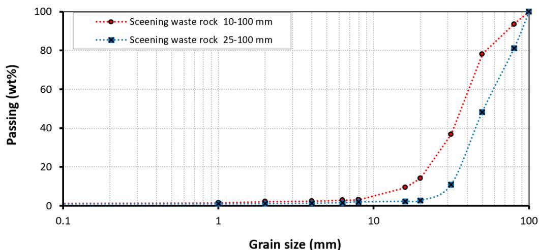
**Figure 4.** Particle size distribution of both 10–100 mm and 25–100 mm aggregate gradations.
