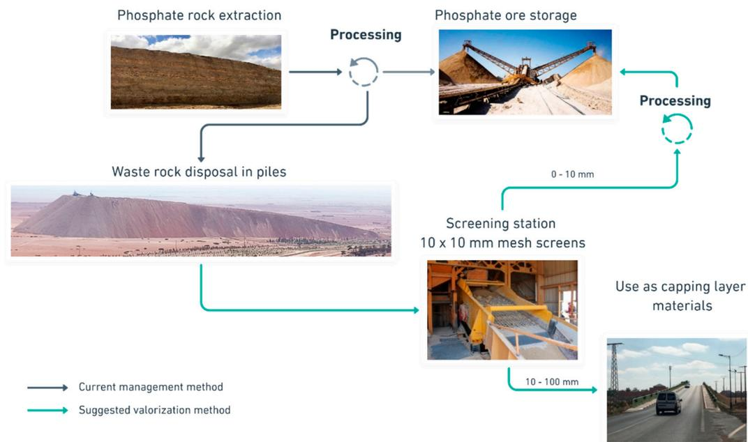
**Figure 8.** From a traditional linear consumption model to a circular phosphate economy: the case of screening waste rock for capping layer applications and lost phosphate recovery.
