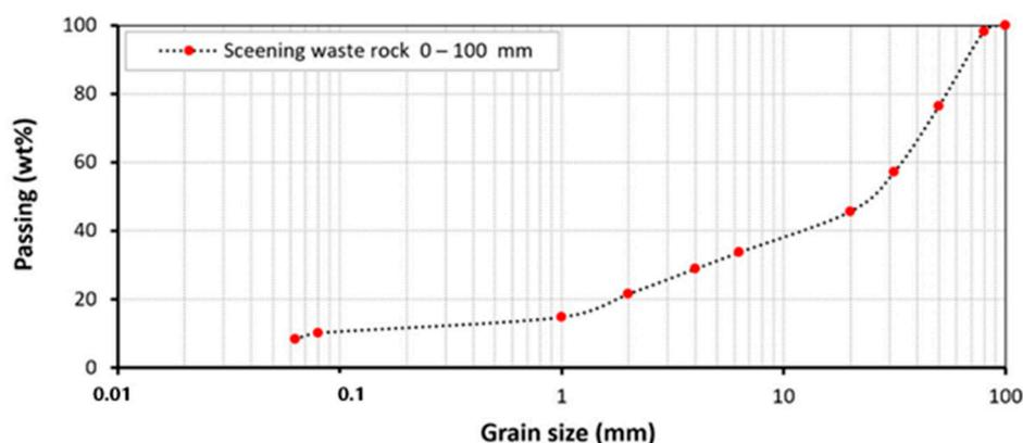
**Figure 3.** Particle size distribution curve of SWR materials.
