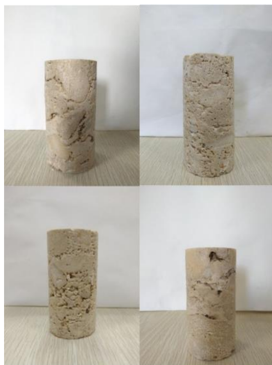
Figure 3. Saturated uniaxial compression specimen.
