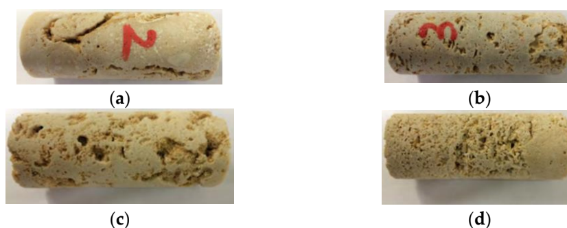
Figure 2. Coral reef limestone grain and structure type. (a) Block structure coral-reef limestone, (b) gravel structure coral-reef limestone, (c) gravel debris structure coral-reef limestone, and (d) sandy debris coral-reef limestone.
