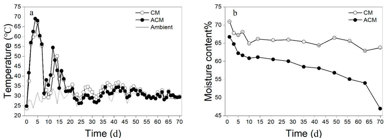
**Figure 3.** Changes in temperature (a) and moisture content (b) in different treatments during composting.
