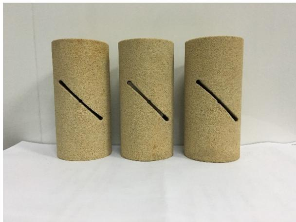
**Figure 1.** Prefabricated fractures in rock samples.
