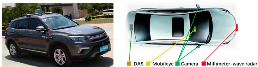
**Figure 1.** Diagram illustrating the equipment installation.
