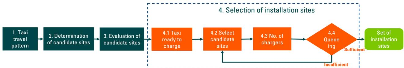
**Figure 1.** Process of analysis of charging station locations.
