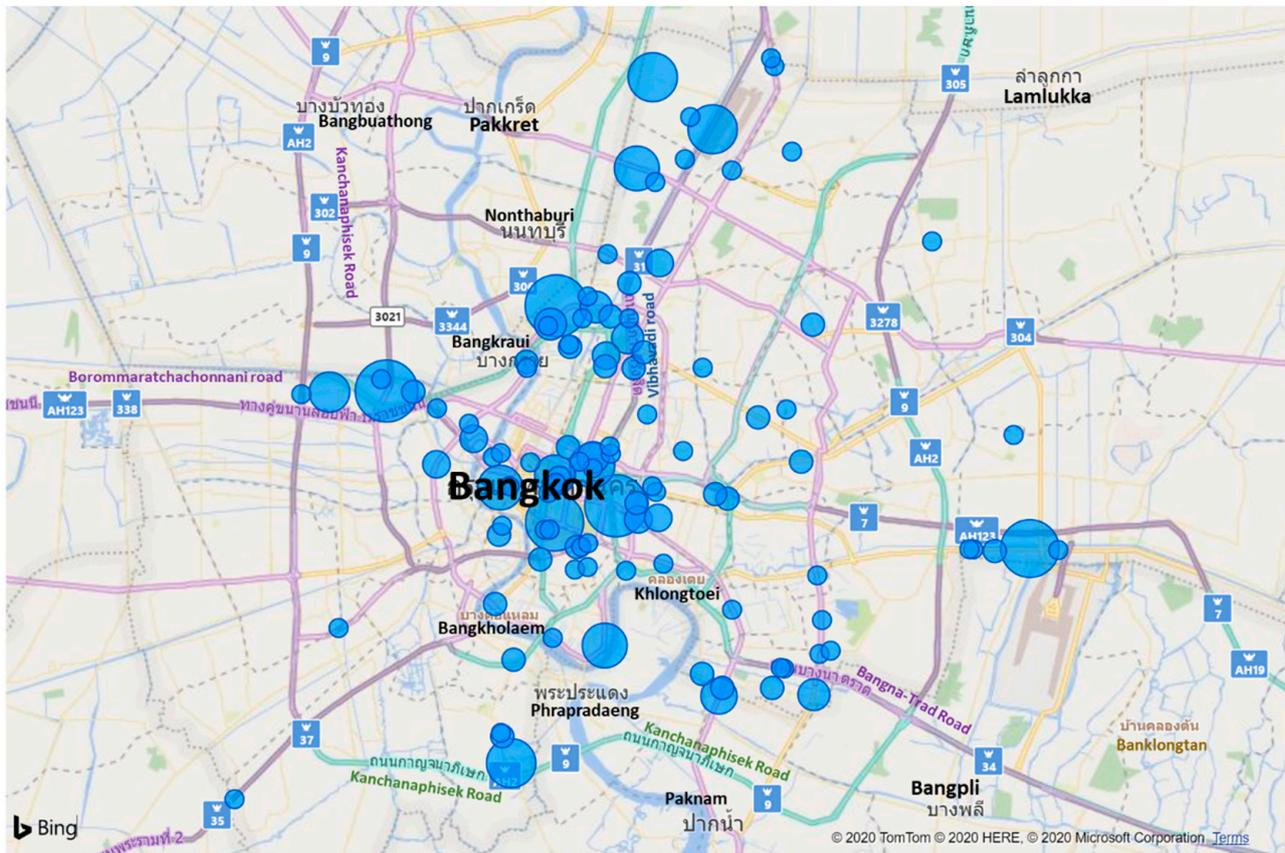
Figure 10. Charging locations to serve BEV taxis based on data from 21 November 2018. Bubble size indicates how many taxis need to charge at the station.
