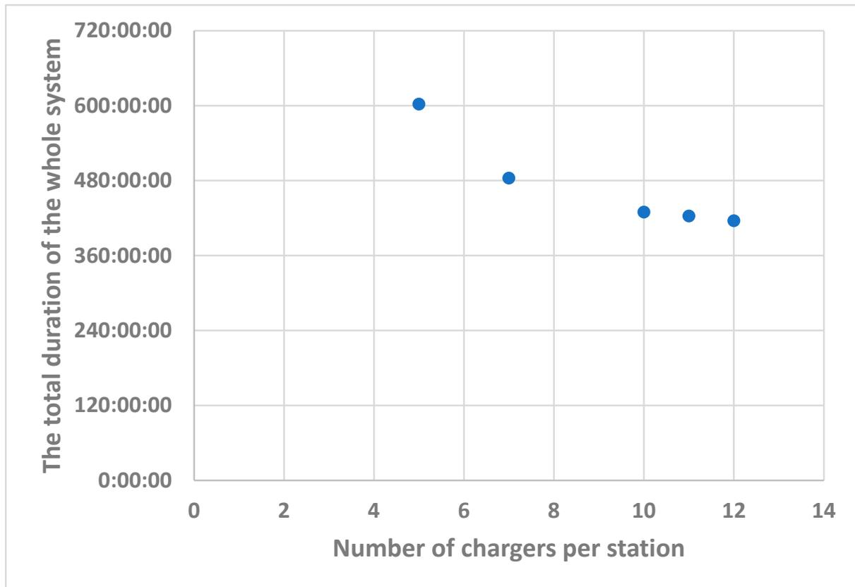
**Figure 9.** Relationship between the number of chargers per station and the total charging time of the system.
