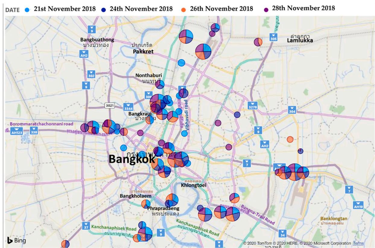
**Figure 11.** Optimal charging station locations based on data from 21 November, 24 November, 26 November, and 28 November 2018.
