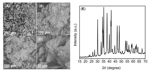
**Figure 5.** SEM images (**A–D**) and XRD diffractogram (**E**) of the powder obtained for 6 w/w% NaOH.
