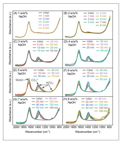
**Figure 4.** FTIR spectra of CO<sub>2</sub> absorption in NaOH solutions with time for (**A**) 1 w/w%; (**B**) 2 w/w%; (**C**) 3 w/w%; (**D**) 4 w/w%; (**E**) 5 w/w%; (**F**) 6 w/w%; (**G**) 7 w/w%; (**H**) 8 w/w%.
