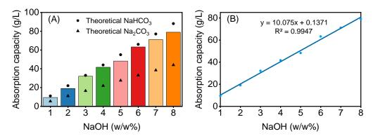
**Figure 8.** (A) Obtained and theoretical absorption capacities for NaOH solutions of 1 to 8 w/w% NaOH. A total conversion of  $CO_2$  to carbonate and bicarbonate ions was assumed to estimate the theoretical capacities using Equations (1) and (2). (B) Linear regression based on the experimental data, indicating that the concentration of NaOH and the absorption capacity correlate linearly.
