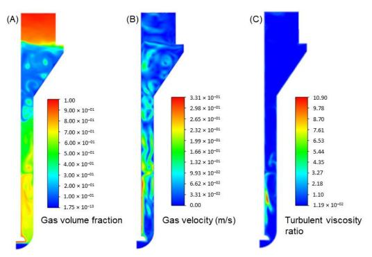
**Figure 3.** Contour plots of the gas volume fraction (**A**), gas velocity (**B**) and turbulent viscosity ratio (**C**) obtained from the CFD simulations.
