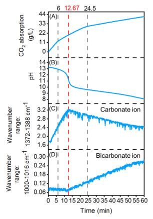
**Figure 6.** CO<sub>2</sub> absorption (**A**), pH (**B**), the sum of the absorbance intensities of the wavenumber range 1372–1388 cm<sup>-1</sup> corresponding to the carbonate ion region (**C**) and the sum of the absorbance intensity of the wavenumber range 1000–1016 cm<sup>-1</sup> corresponding to the bicarbonate ion region (**D**) with time for 4 w/w % NaOH.
