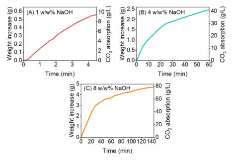
**Figure 7.** Weight increase of the reactor and the corresponding CO<sub>2</sub> absorption for 1 (**A**), 4 (**B**) and 8 (**C**) w/w% NaOH.
