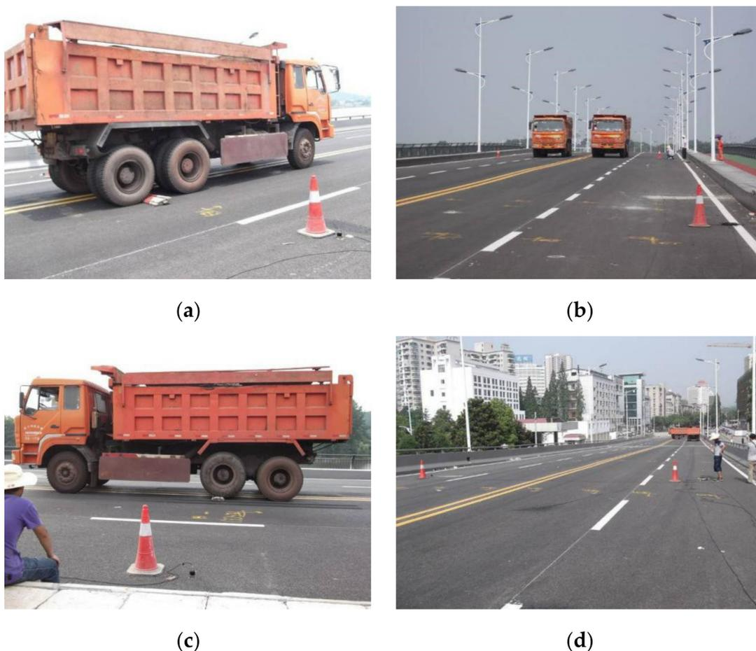
**Figure 12.** Bridge load test. (a) Jumping test; (b) Sporting test; (c) Braking test; (d) Pulsation test.
