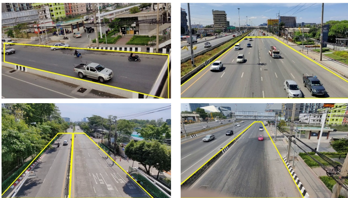
Figure 35. Output images with road boundaries using the improved RLB-CCTV algorithm.
