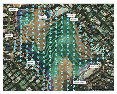
Figure 5. UAV's flight plan.
