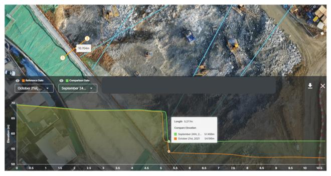
Figure 8. Height difference and slope monitoring of segment of interest.
