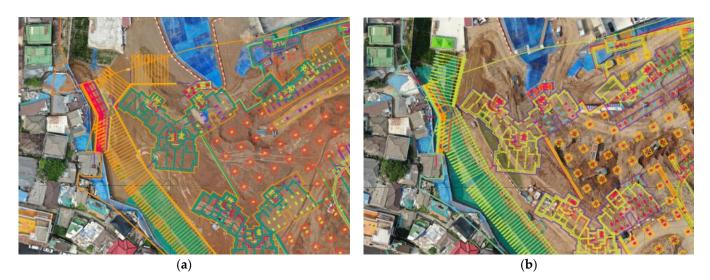
**Figure 9.** Site monitoring using UAV aerial photograph: (**a**) initial design of ground anchor; (**b**) changed design of ground anchor.
