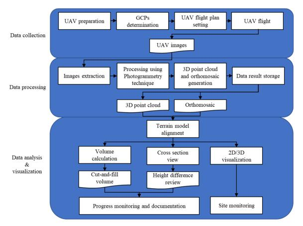
Figure 4. UAV-based earthwork management framework.
