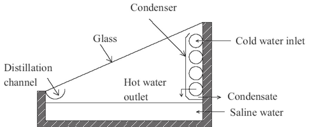
**Figure 22.** Solar still coupled with an internal condenser (Khalifa et al. [96], “Reprinted/adapted with permission from Ref. [96]. 1999, Elsevier”).
