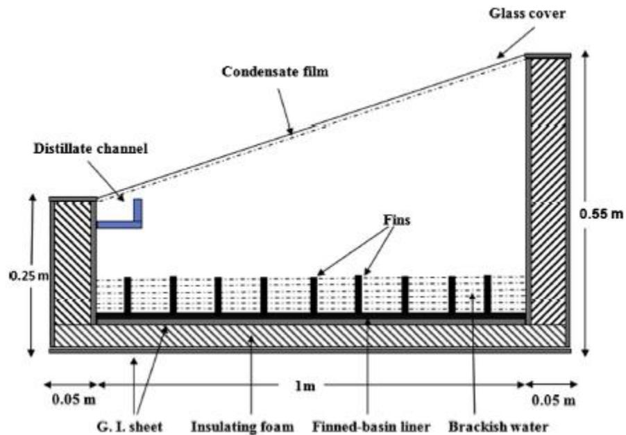
**Figure 12.** Sketch of the fin-type solar still (El-Sebail and El-Naggar [58], “Reprinted/adapted with permission from Ref. [58]. 2017, Elsevier”).
