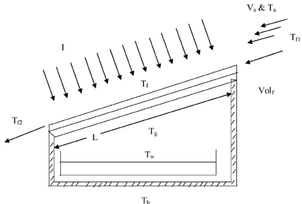
Figure 6. Schematic of water film solar still (Mousa and Bassam [36], “Reprinted/adapted with permission from Ref. [36]. 1997, Elsevier”).
