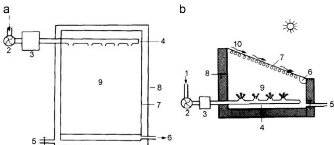
**Figure 43.** Diagrammatic representation of air-bubbled solar still (a) top view, (b) side view (Pandey [139], “Reprinted/adapted with permission from Ref. [139]. 1984, Elsevier”).
