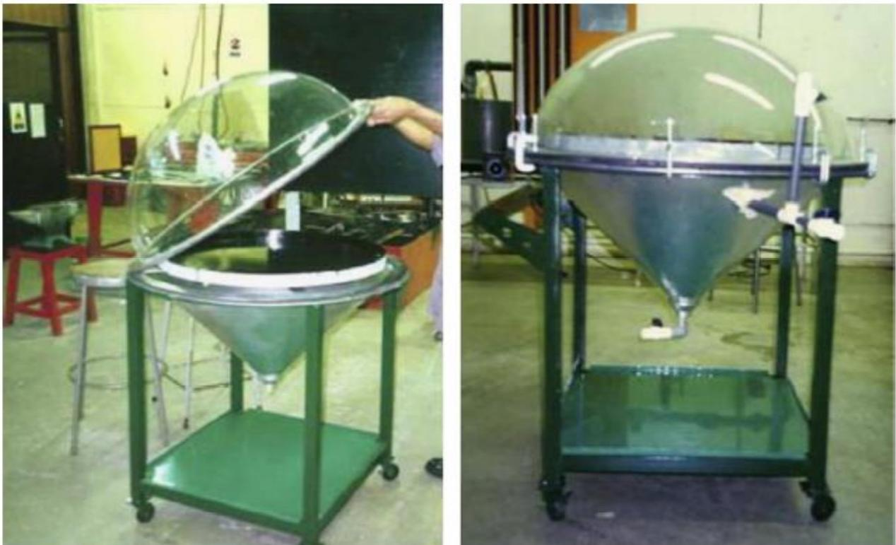
Figure 30. Photo of the hemispherical solar still (Ismail [112], “Reprinted/adapted with permission from Ref. [112]. 2009, Elsevier”).
