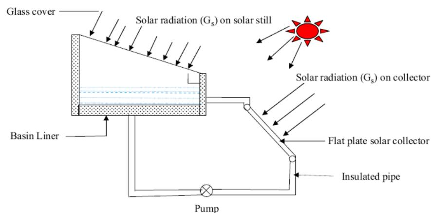
**Figure 13.** Sketch of the solar still integrated with a flat plate solar collector (Ranjan and Kaushik [16], “Reprinted/adapted with permission from Ref. [16]. 2013, Elsevier”).
