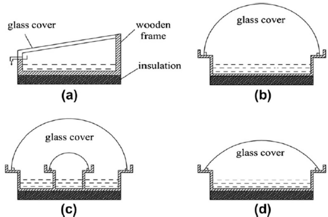
**Figure 2.** Sketch of the conventional basin solar stills with different glass covers (Tayeb [23], “Reprinted/adapted with permission from Ref. [23]. 1992, Elsevier”). (a) Sloped flat cover, (b) Half cylinder cover, (c) Two half cylinders cover, (d) Slightly curved cover.
