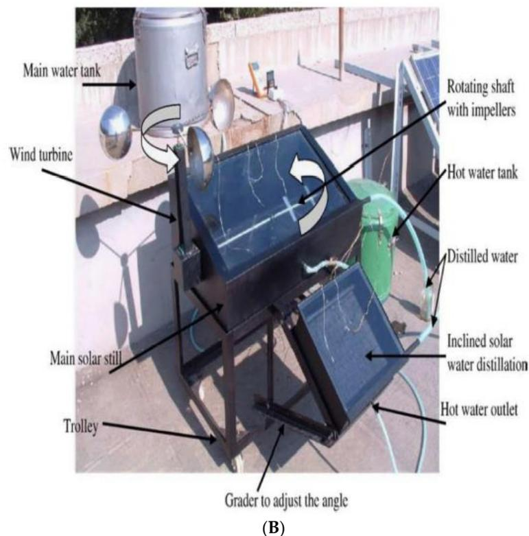
**Figure 33.** Schematic diagram and photo of the rotating shaft solar still. (A). Abdel-Rehim and Lasheen [123], “Reprinted/adapted with permission from Ref. [123]. 2005, Elsevier”. (B). Eltawil and Zhengming [124], “Reprinted/adapted with permission from Ref. [124]. 2009, Elsevier”.
