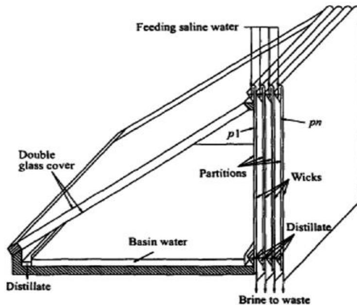
**Figure 41.** Schematic diagram of basin-multiple-effect diffusion coupled solar still (Tanaka et al. [136], “Reprinted/adapted with permission from Ref. [136]. 2002, Elsevier”).
