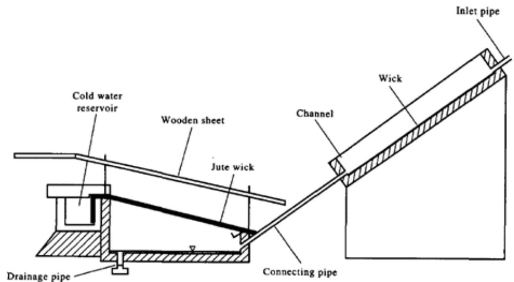
**Figure 18.** Schematic diagram of the wick-basin solar still (Minasian and Al-Karaghoulouli [88], “Reprinted/adapted with permission from Ref. [88]. 1994, Elsevier”).
