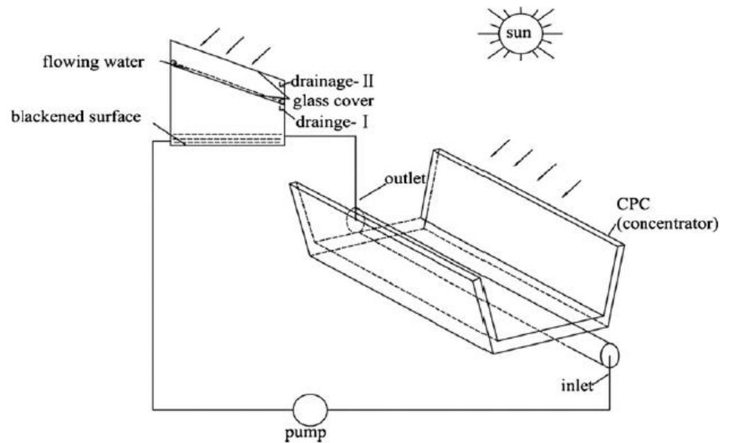
**Figure 14.** Sketch of the solar still integrated with a (CPC) collector (Tanaka [63], “Reprinted/adapted with permission from Ref. [63]. 2011, Elsevier”).
