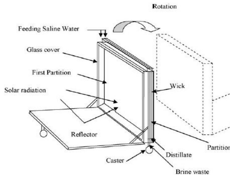
**Figure 7.** Multiple effect diffusion solar still (Tanaka et al. [39], “Reprinted/adapted with permission from Ref. [39]. 2000, Elsevier”).
