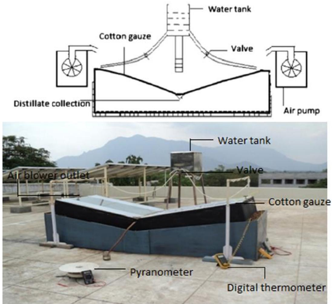
Figure 39. Schematic diagram and photo of V-type solar still (Suneesh et al. [133], “Reprinted/adapted with permission from Ref. [133]. 2014, Elsevier”).
