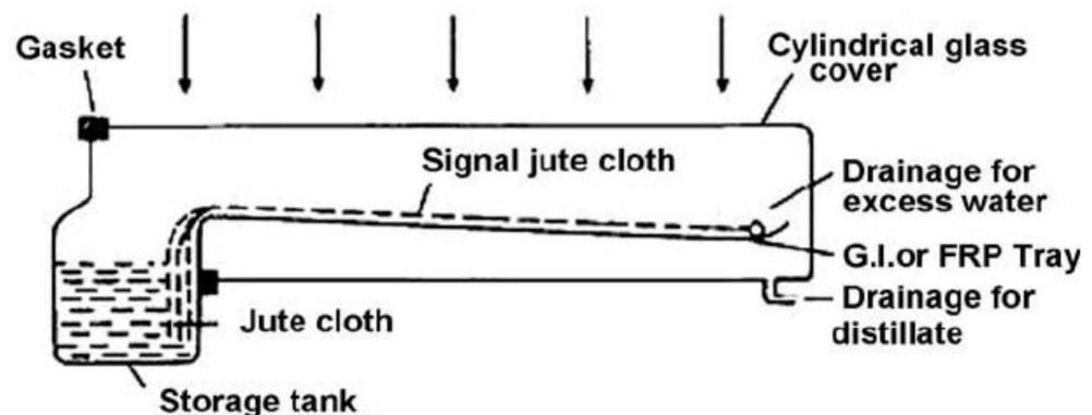
Figure 27. Diagrammatic representation of the tubular multi-wick solar still (Ashok and Anand [109], “Reprinted/adapted with permission from Ref. [109]. 1992, Elsevier”).
