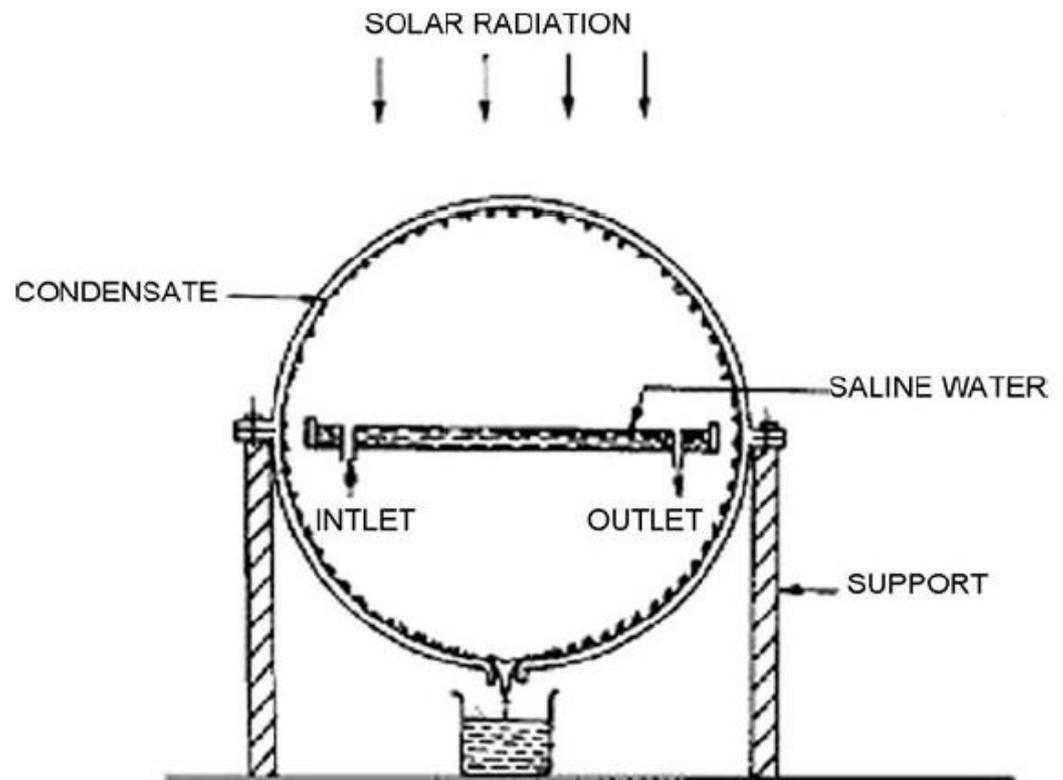
**Figure 28.** Schematic diagram of the spherical solar still (Dhiman [110], “Reprinted/adapted with permission from Ref. [110]. 1988, Elsevier”).
