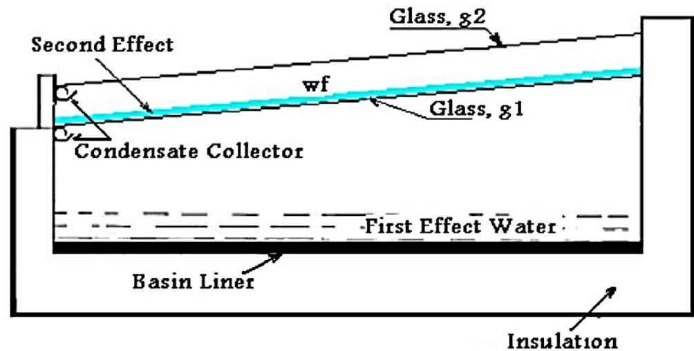
Figure 9. Sketch of the regenerative solar still (Zurigat and Abu-Arabi [48], “Reprinted/adapted with permission from Ref. [48]. 2004, Elsevier”).
