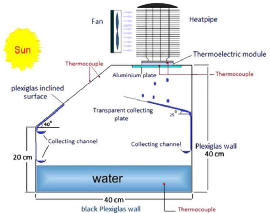
**Figure 38.** Diagrammatic representation of the thermoelectric solar still (Rahbar and Esfahani [132], “Reprinted/adapted with permission from Ref. [132]. 2012, Elsevier”).
