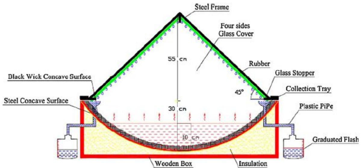
**Figure 17.** Schematic diagram of concave wick surface solar still (Kabeel [86], “Reprinted/adapted with permission from Ref. [86]. 2009, Elsevier”).
