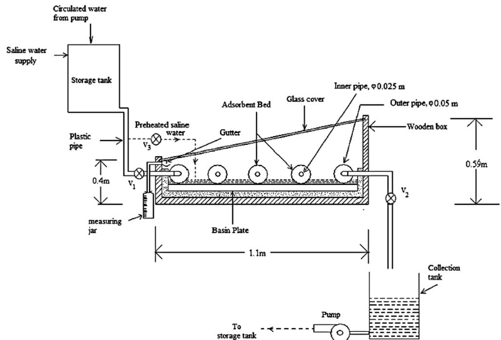
**Figure 35.** Schematic diagram of the vapor adsorption solar still (Kannan et al. [128], “Reprinted/adapted with permission from Ref. [128]. 2014, Elsevier”).
