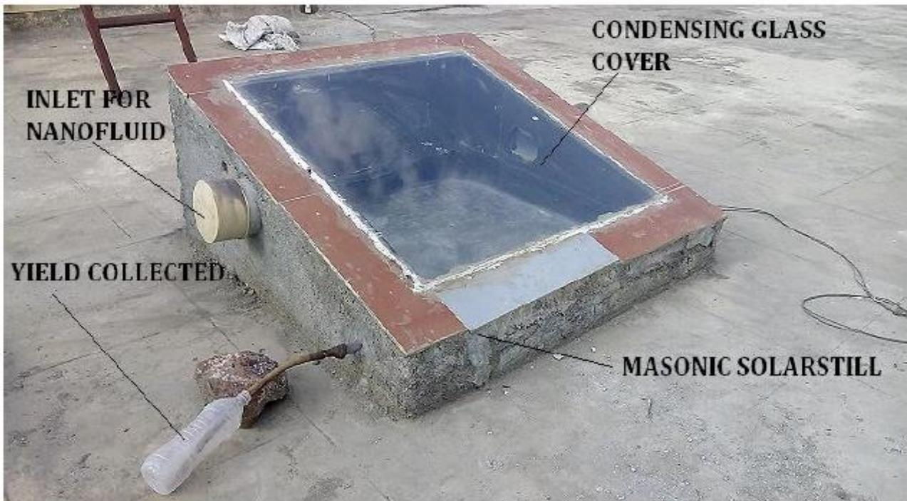
Figure 36. Photo of the masonic solar still (Navale et al. [130], “Reprinted/adapted with permission from Ref. [130]. 2016, Elsevier”).
