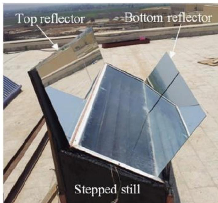
**Figure 20.** Stepped solar still with internal and external reflectors (Omara et al. [92], “Reprinted/adapted with permission from Ref. [92]. 2014, Elsevier”).
