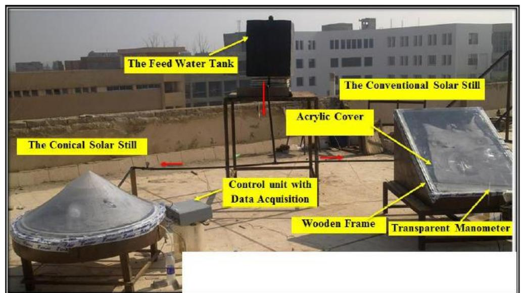
**Figure 34.** Schematic diagram and photo of the conical solar still (Gad et al. [127], “Reprinted/adapted with permission from Ref. [127]. 2015, Elsevier”).
