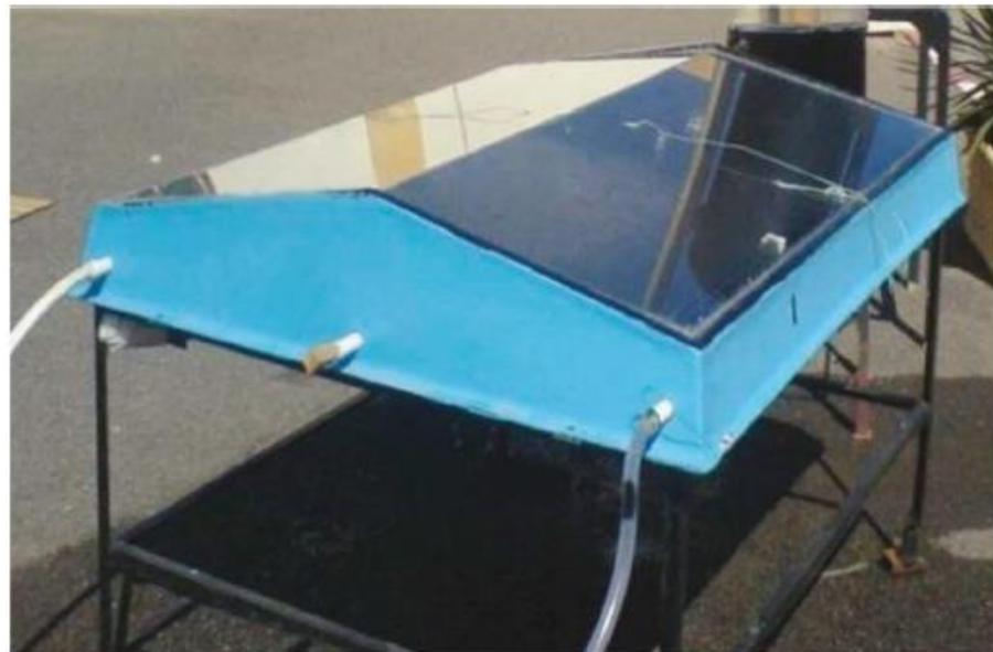
**Figure 4.** Sketch and photo of the double slope basin solar still. (A). El-Maghlany [30], “Reprinted/adapted with permission from Ref. [30]. 2012, Elsevier”. (B). Hanane et al. [31], “Reprinted/adapted with permission from Ref. [31]. 2002, Elsevier”.
