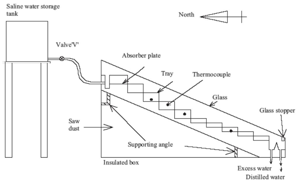
**Figure 19.** Schematic diagram of stepped solar still (Velmurugan et al. [89], “Reprinted/adapted with permission from Ref. [89]. 2009, Elsevier”).
