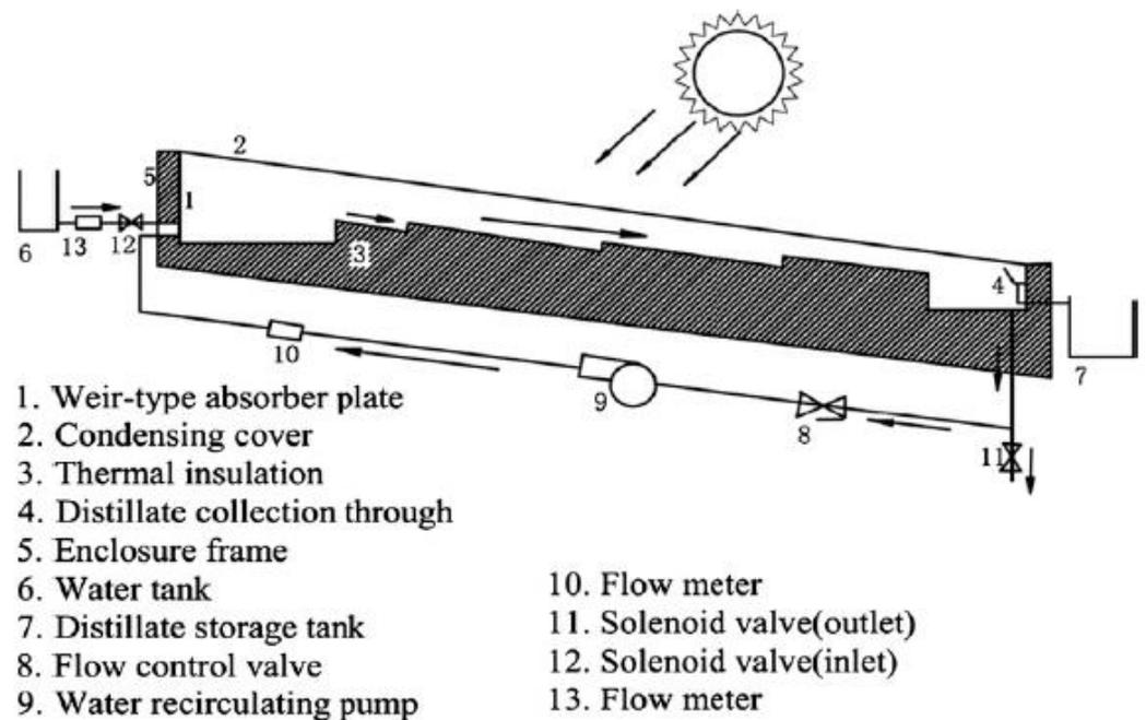
**Figure 23.** Schematic of a weir-type solar still (Sadineni et al. [98], “Reprinted/adapted with permission from Ref. [98]. 2008, Elsevier”).
