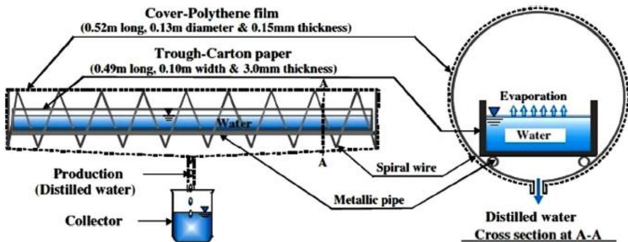
Figure 26. Schematic diagram of the tubular solar still (Amimul et al. [106], “Reprinted/adapted with permission from Ref. [106]. 2012, Elsevier”).
