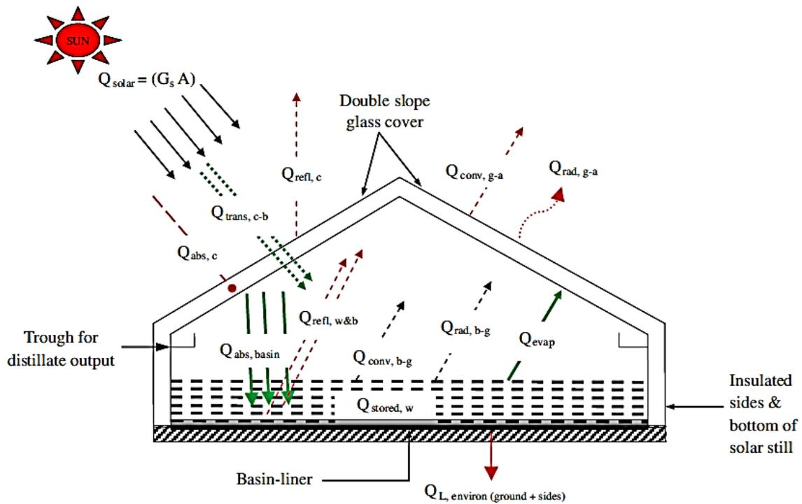
Figure 5. Heat transfer in a double-slope basin solar still (Ranjan and Kaushik [16], “Reprinted/adapted with permission from Ref. [16]. 2013, Elsevier”).
