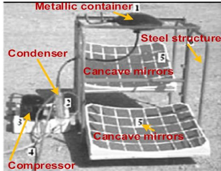
**Figure 42.** Photo of the point focus elliptical shape solar still (Nassar et al. [138], “Reprinted/adapted with permission from Ref. [138]. 1984, Elsevier”). (1) container, (2) condenser, (3) compressor, (4) flexible tube, (5) concave mirrors.
