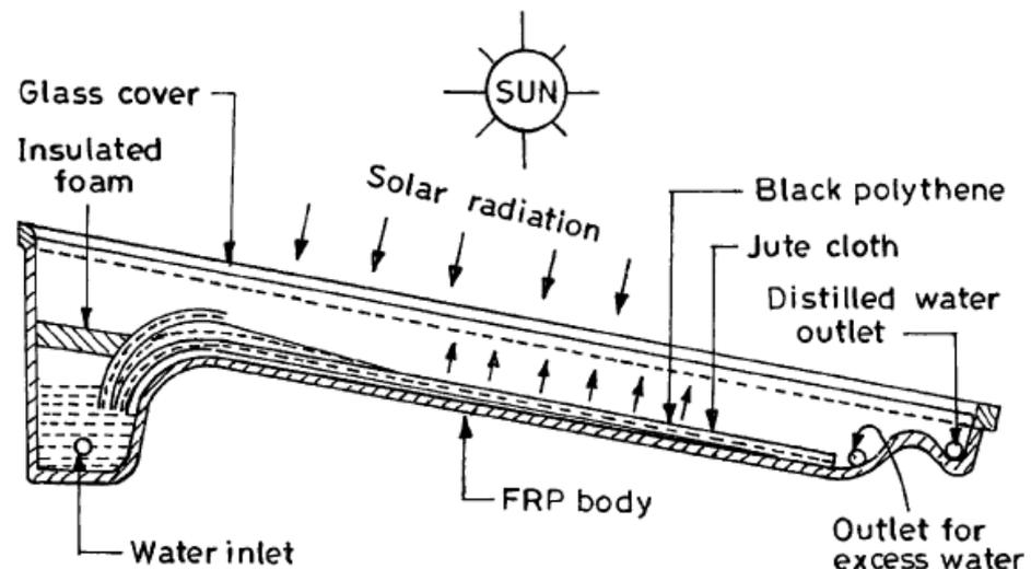
**Figure 16.** Cross-section of FRP multi-wick solar still (Tiwari et al. [9], “Reprinted/adapted with permission from Ref. [9]. 2003, Elsevier”).
