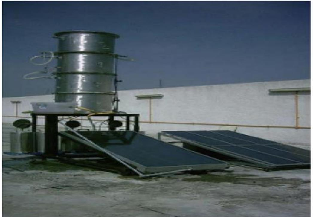
**Figure 40.** Schematic diagram and photo of multistage evacuated solar still (Ahmed et al. [135], “Reprinted/adapted with permission from Ref. [135]. 2009, Elsevier”).
