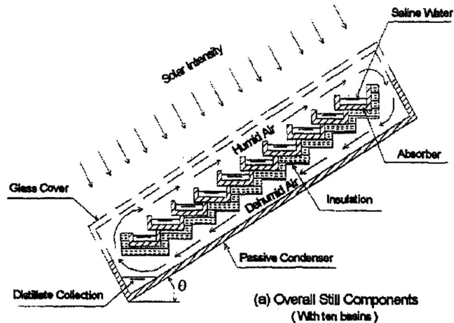
Figure 37. Schematic diagram of the humidifier-dehumidifier solar still (Fath et al. [131], “Reprinted/adapted with permission from Ref. [131]. 2003, Elsevier”).
