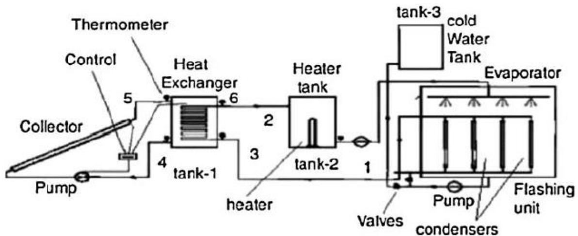
Figure 29. Diagrammatic representation of the multi-effect solar still (Abdel Dayem [111], “Reprinted/adapted with permission from Ref. [111]. 2006, Elsevier”).
