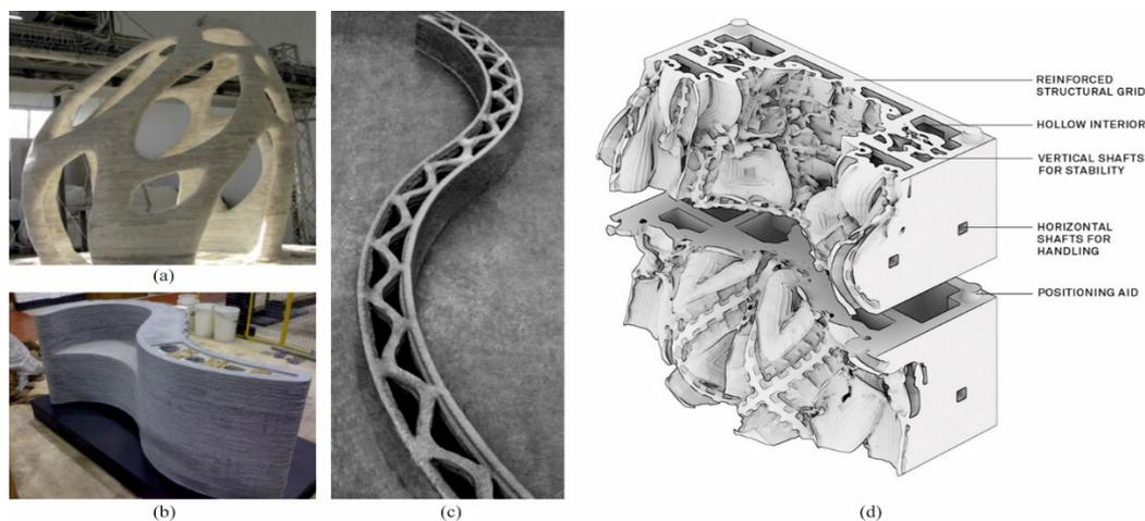
**Figure 5.** Full-scale printed structures through (a) D-shape printing, (b) concrete printing, (c) contour crafting process [43], and (d) printed digital grotesque [48].
