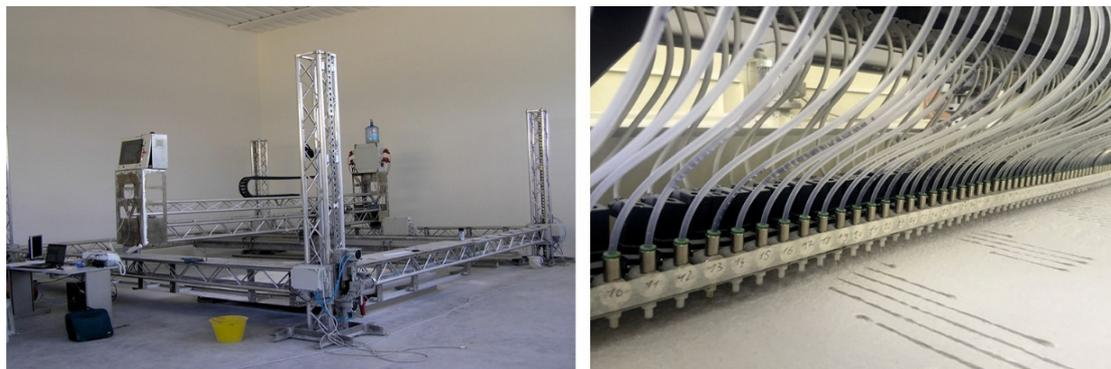
**Figure 4.** D-shape 3D printer with 300 nozzles (left), and print head (right) [48,49].
