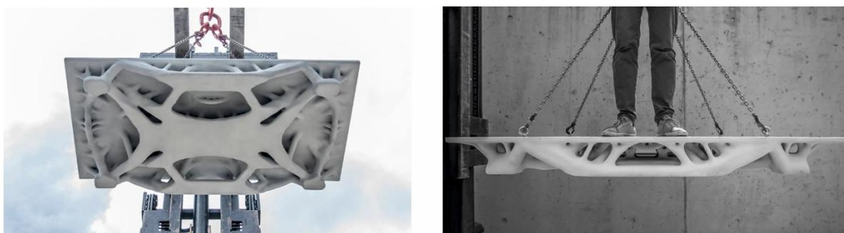
**Figure 13.** 3D-printed prototype of CSC slab (Digital Building Technologies, ETH Zurich, Switzerland) [193].
