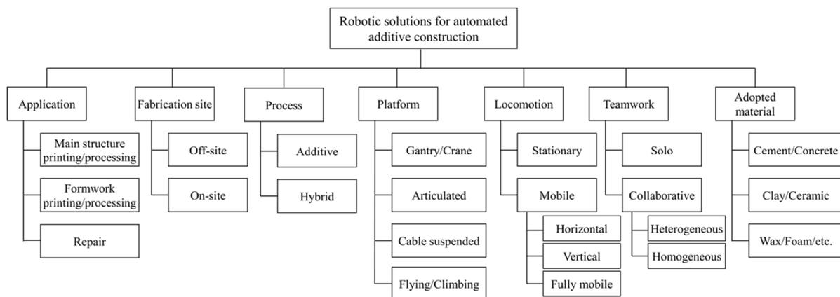
**Figure 7.** Categories and different aspects of the adopted robotic solutions for automated additive construction.
