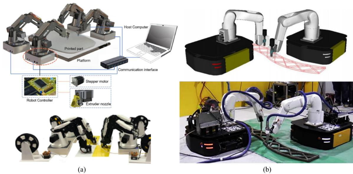
**Figure 12.** Developed multi-robot 3D printing system by (a) Shen et al. [140] with stationary robots, and (b) Zhang et al. [126] with mobile robots.
