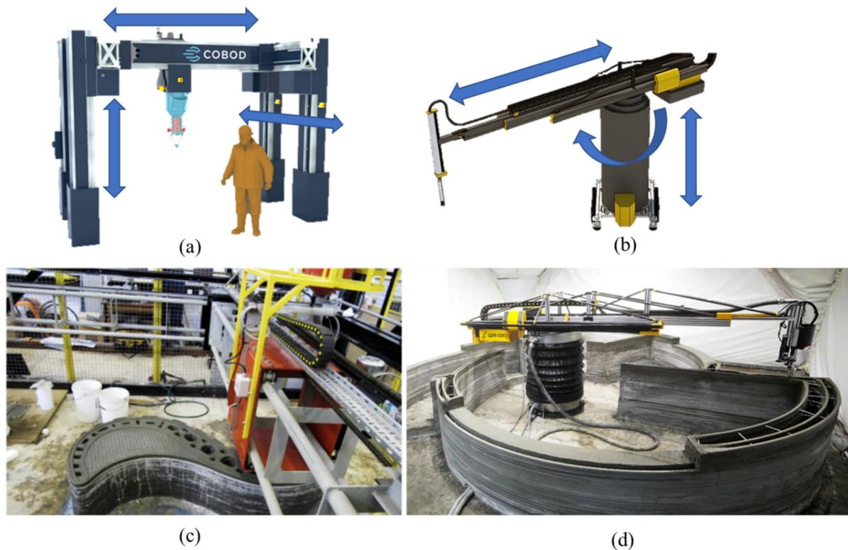
**Figure 8.** Gantry and crane robots for large-scale AM (a) illustration of a gantry robot printer and its three axes—COBOD [94,95], (b) illustration of a crane robot printer and its three axes—ApisCor [96], (c) concrete printing using a gantry robot [37], and (d) concrete printing using an ApisCor crane robot [94,96].
