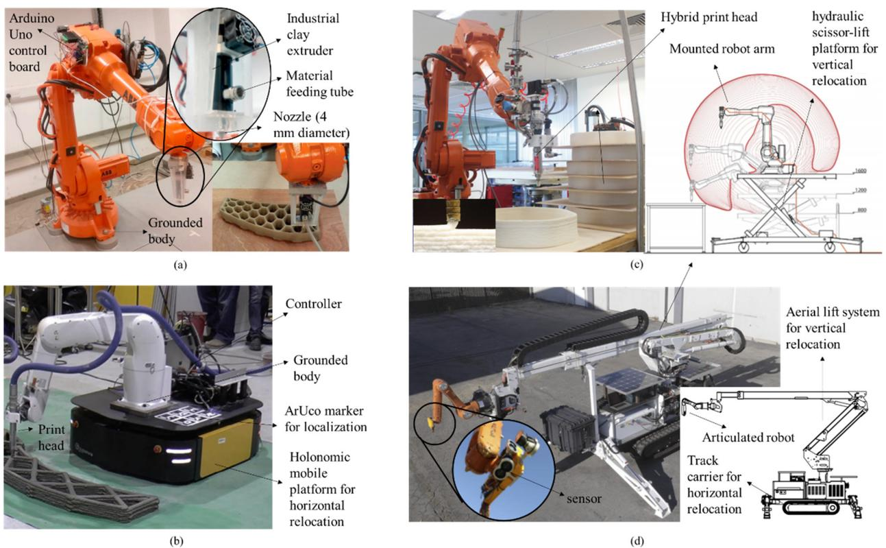
**Figure 10.** Different categories of articulated robots for large-scale AM (a) stationary articulated robots [131], (b) horizontally mobile articulated robots [126], (c) vertically mobile articulated robots [132], and (d) both horizontally and vertically mobile articulated robots [124].
