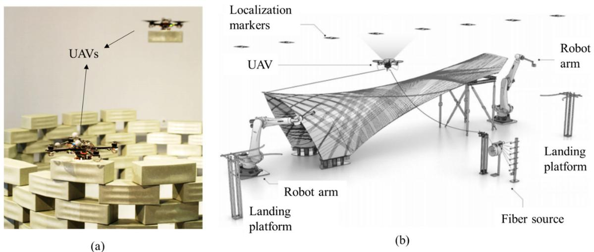
**Figure 11.** Illustrations of different categories of multi-robot solutions for non-AM based construction (a) homogenous, i.e., uniform entities [135], and (b) heterogeneous, i.e., diverse entities [139].
