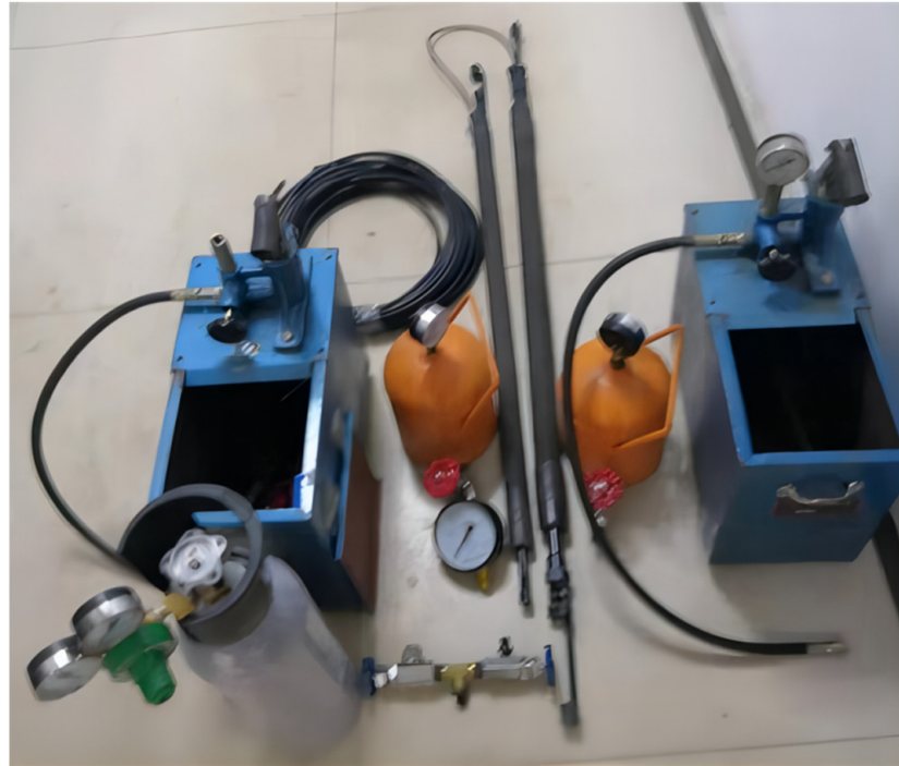
Figure 11. Physical photo of hole sealing device.
