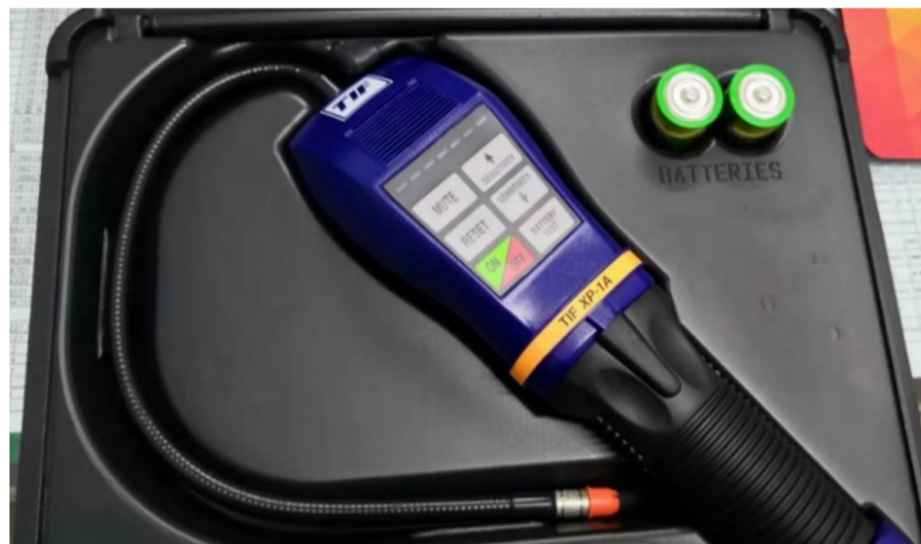
Figure 12. XP-1A qualitative leak detector.
