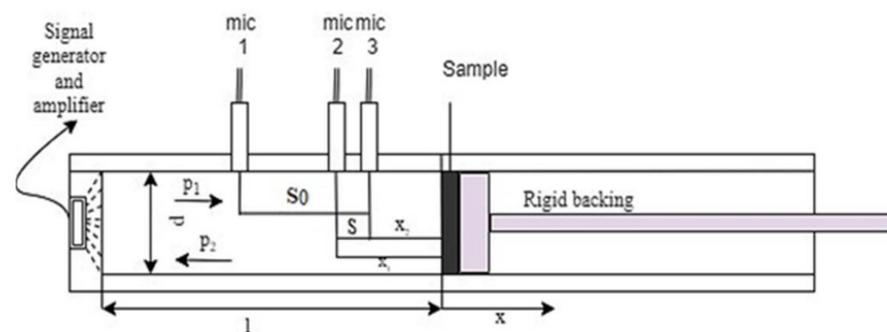
**Figure 2.** Impedance tube setup.
