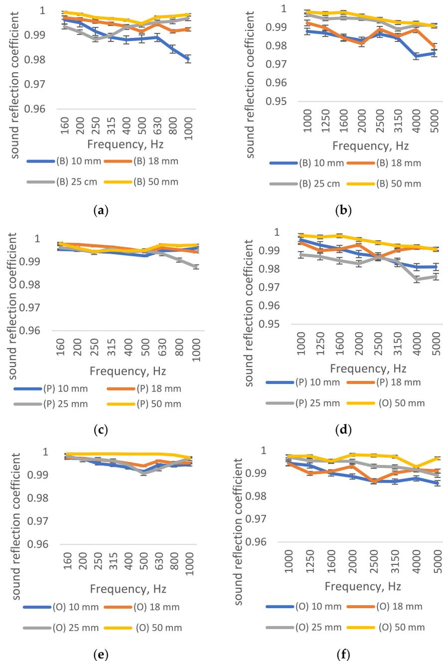
**Figure 4.** Sound reflection coefficient measurements using impedance tube: (a) birch at 160–1000 Hz; (b) birch at 1250–5000 Hz; (c) pine at 160–1000 Hz; (d) pine at 1250–5000 Hz; (e) oak at 160–1000 Hz; (f) oak at 1250–5000 Hz.
