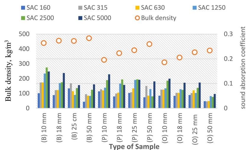
**Figure 3.** Influence of charcoal thicknesses and densities on sound absorption coefficient (SAC) at 160 Hz, 315 Hz, 630 Hz, 1250 Hz, 2500 Hz, and 5000 Hz in samples with thicknesses of 10 mm, 18 mm, 25 mm, and 50 mm. Types of wood charcoal samples: (O) oak; (B) birch; (P) pine.
