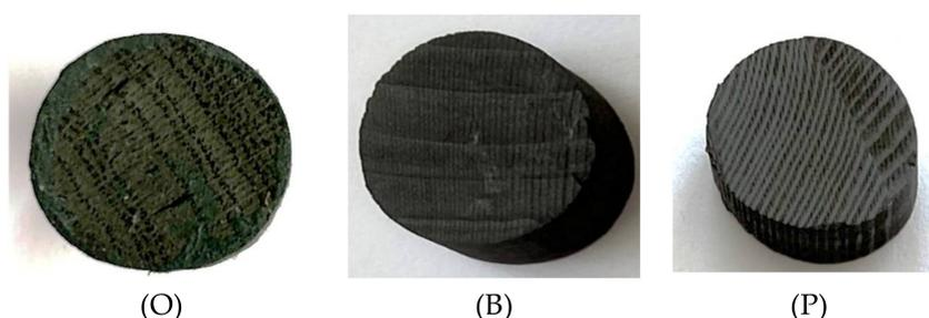
**Figure 1.** Different types of wood charcoal samples: (O) oak; (B) birch; (P) pine.
