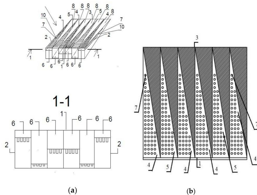
**Figure 5.** Acoustic diffuser: (a) top view; (b) exploded view.
