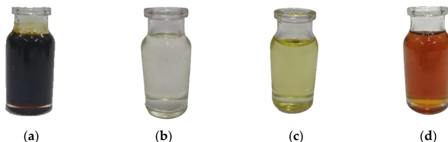
**Figure 6.** Color and visual appearance of pyrolytic oil obtained from (a) mixed plastic waste, fractionation of mixed plastic waste at (b) 150 °C (light), (c) 320 °C (medium), and (d) 460 °C (heavy).
