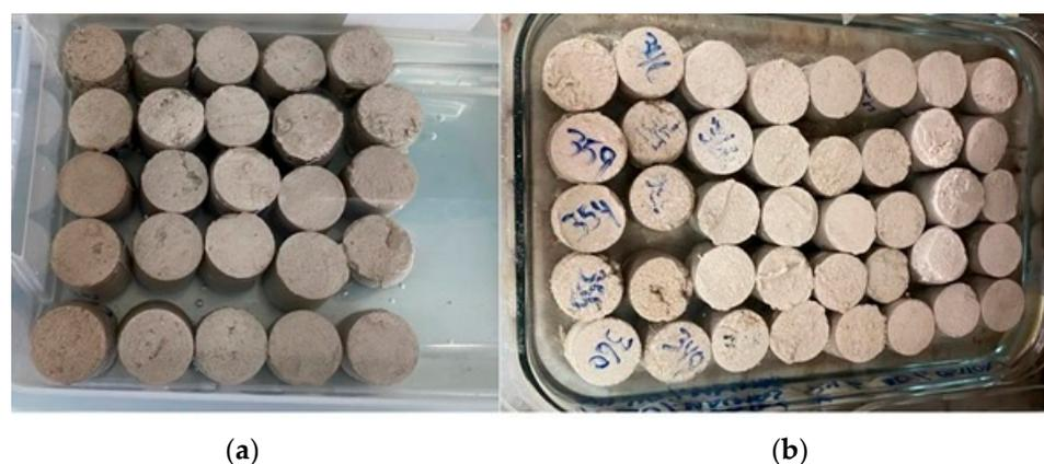
**Figure 3.** Submerged samples during (a) water immersion and (b) acid immersion.
