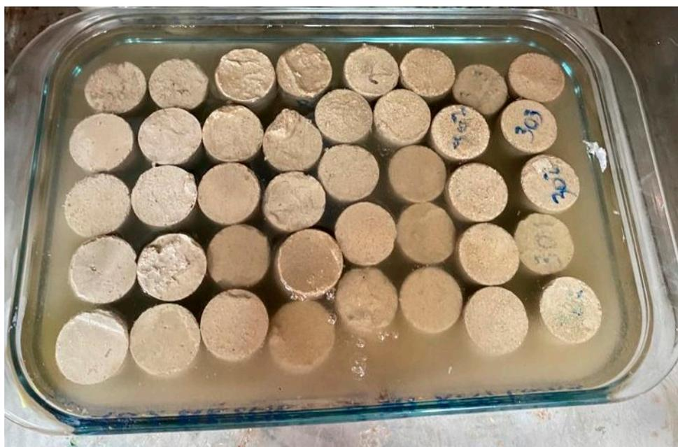
**Figure 4.** Samples were submerged in sulfate salts.
