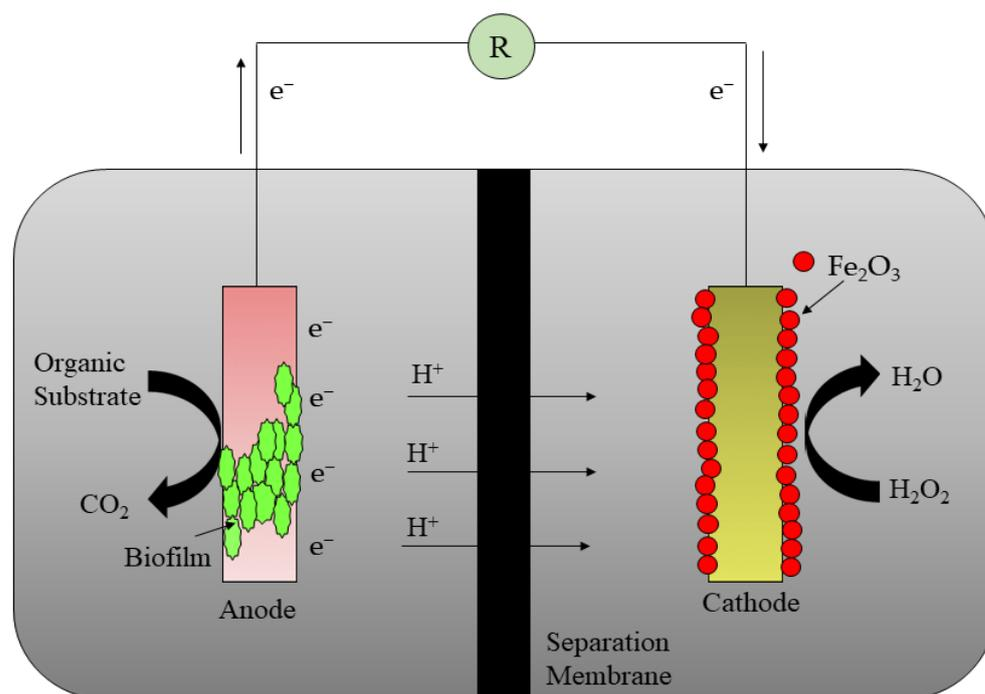
**Figure 2.** Schematic representation of the MFC–Fenton system.
