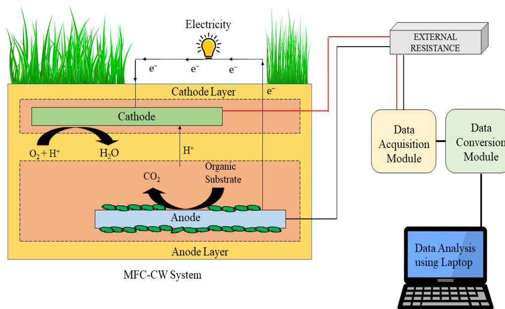
**Figure 1.** Schematic of an MFC-constructed wetland system for the degradation of antibiotics.
