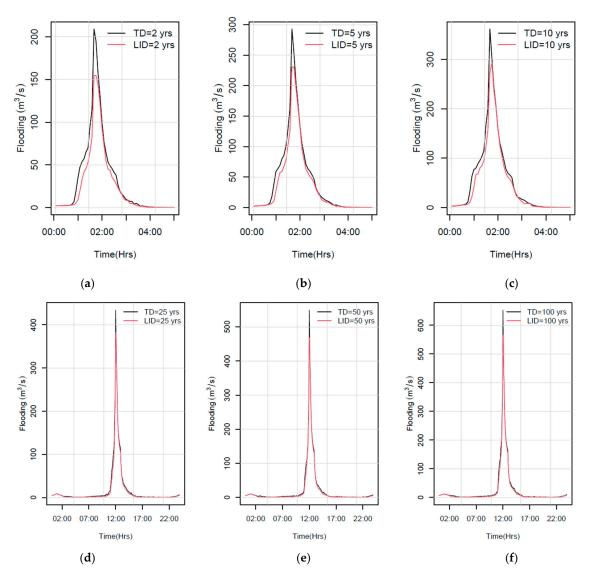
**Figure 7.** Peak reduction of the flooding system of events with a typical duration of 200 min: (**a**) 2-year recurrence period; (**b**) 5-year recurrence period; (**c**) 10-year recurrence period. Peak reduction of the flooding system of events with a typical duration of 200 min: (**d**) 25-year recurrence period; (**e**) 50-years recurrence period; (**f**) 100-year recurrence period.
