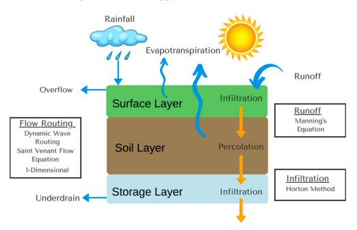
**Figure 2.** Conceptual hydrological process for bio-retention cells in Stormwater Management Model (SWMM).
