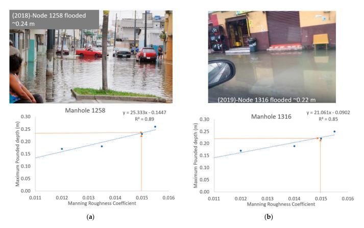
**Figure A5.** Sensitive analyzed to the manning coefficient according to the flooded levels registered on site. On each point, the model ran four times to obtain each referce Manning's value and level of flooding. (a) Point located between the 10 de Agosto Street and Otavalo street. (b) Potin located between Rafael Garcia Goyena street and Avenida 43.
