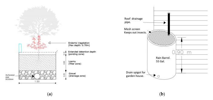
Figure A3. Example of LID applied of the study area: (a) Bioretention cells, and (b) Rain barrels.
