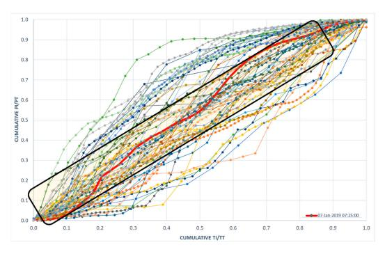
**Figure 4.** 78 normalized storms plotted from March 2018 to July 2019. The typical event is the storm which occurred on January 07 of 2019 (red line) and was registered by the "Pantanos Secos station". It started at 7:25 a.m. and finished at 10:45 a.m. Normalization processes considered accumulative rainfall (PI) and storm duration (TI) to total rainfall (PT) and total duration (TT) respectively.
