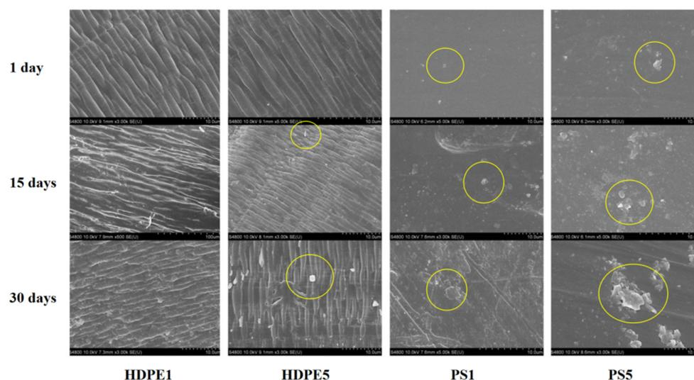
**Figure 2.** SEM images of various MP kinds and concentrations as a function of exposure duration.
