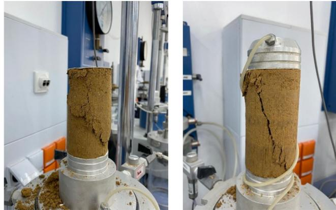
**Figure 7.** Failure planes of soil samples treated with CSA cement.
