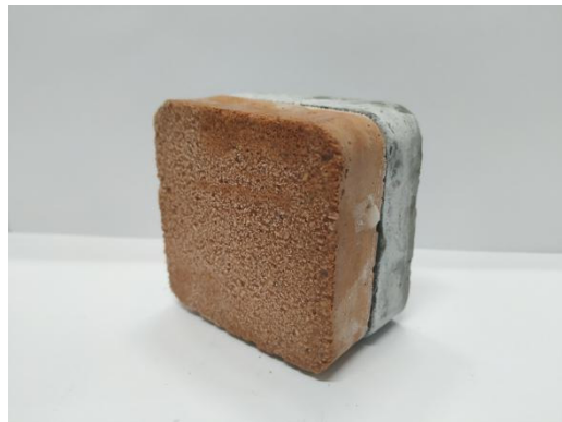
Figure 9. Sample surface after freeze–thaw cycle.
