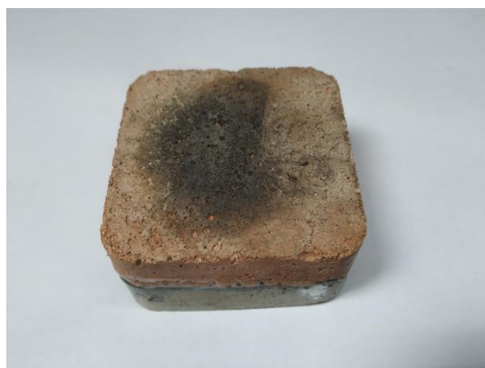
Figure 10. Sample surface after burning.
