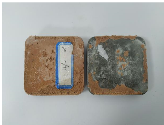
Figure 8. The sample is damaged at the glue joint.
