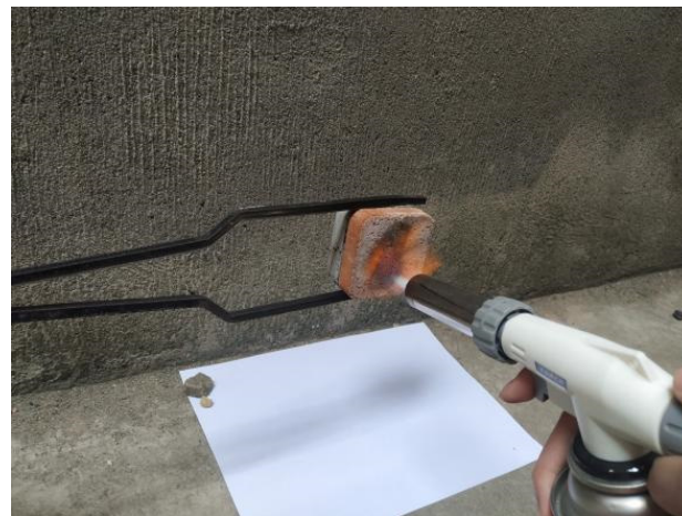
Figure 7. Igniting the surface of the component.
