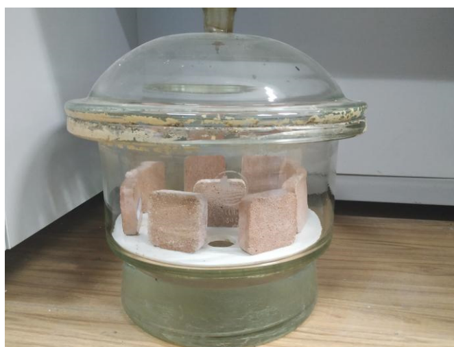
Figure 4. Moisture-proof performance test of composite structure thermal bridge insulation component.
