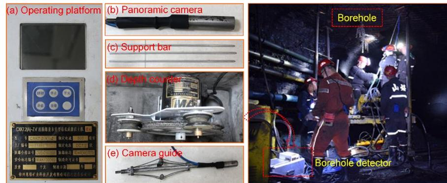
**Figure 12.** Field measurement of borehole television logging for determining the HWCFZ. (a) The operating platform for borehole television logging. (b) The panoramic camera. (c) The support bar to transport the camera to the detection position. (d) The depth counter to measure the distance from the starting point of the drillhole to the detection position. (e) The camera guide to make it easy for the camera to pass through.
