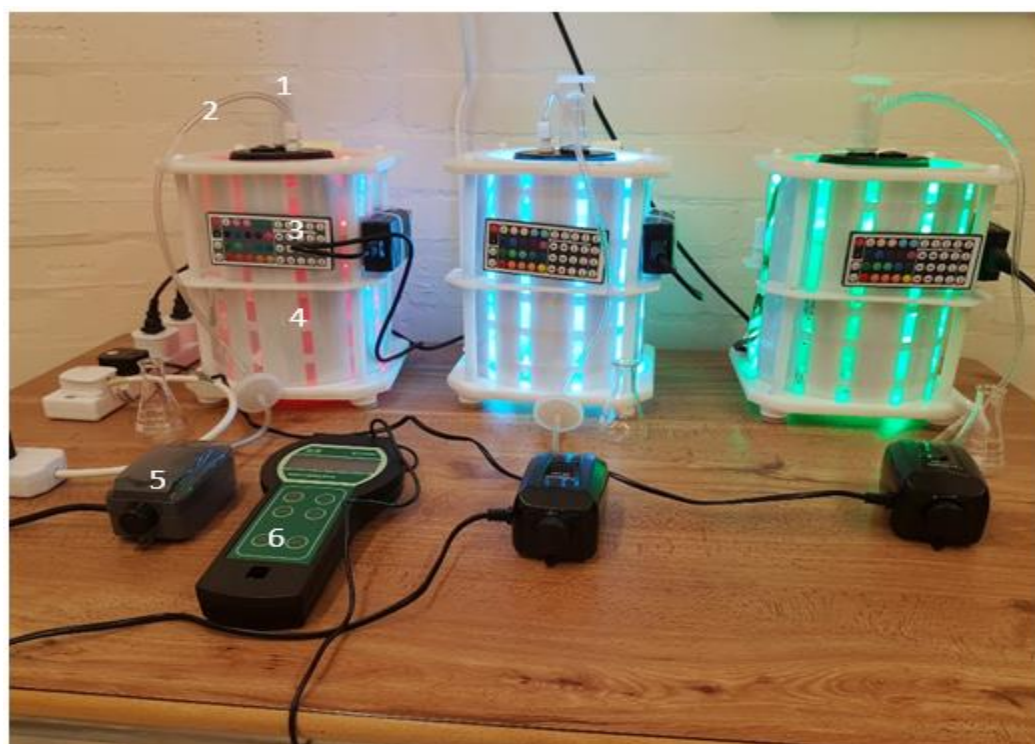
Figure 1. Closed PBR used in this research. (1) Tube head; (2) CO 2 tube; (3) LED lighting remote; (4) PBR outer cover; (5) pump for mixing; (6) handheld photometer.
